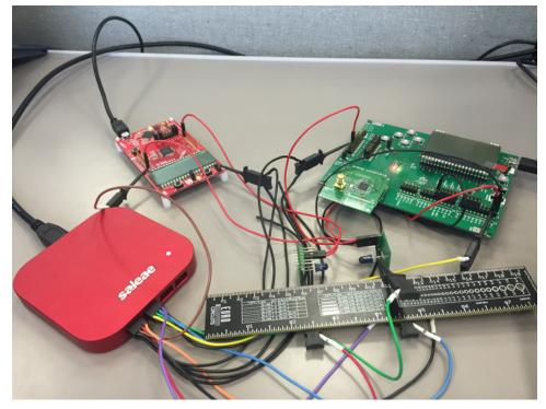
Figure 4. Test Setup With Two TIDA-01212 Boards "Face-to-Face" (TX and RX)
