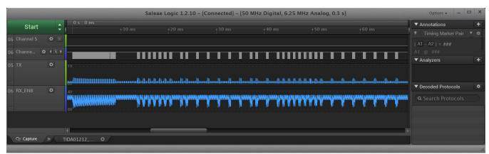
Figure 11. IR Input Signal From TV RC Using NEC IR Protocol
