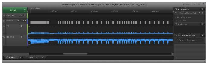
Figure 12. RX\_ENB is the Analog Signal Input to COMPA (Using an Internal Reference of DCOUPL = 1.27 V)
