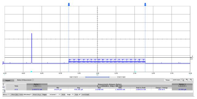
Figure 17. RF Transmission Pulse, Sleep Mode, and LCD Activity With TIDA-00848+TIDA-01212
