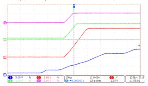
Figure 13. Power Supply Start-Up
