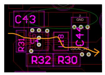
Figure 18. Step-Down Switched-Mode Power Supply Routing
