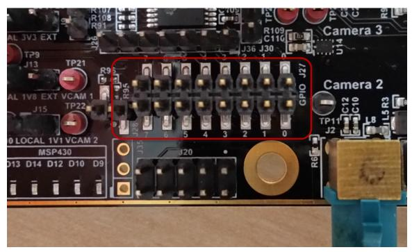
Figure 9. GPIO Jumpers
