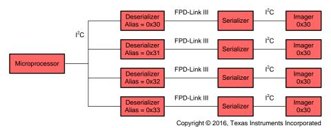
Figure 4. I<sup>2</sup>C Address Aliasing
