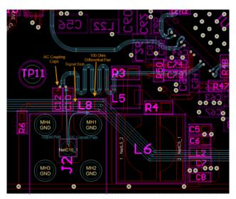
Figure 20. LVDS Signal Pair Routing
