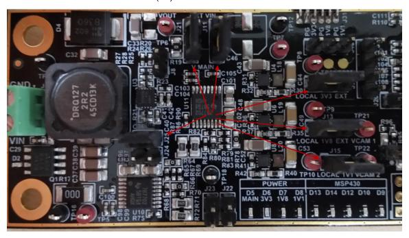
Figure 8. Power Supply Jumpers
