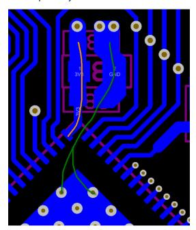
Figure 19. Decoupling Current Loop
