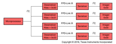
Figure 15. I<sup>2</sup>C Address Aliasing
