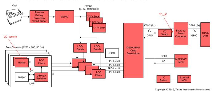
Figure 12. Setup for Monitoring I<sup>2</sup>C Transactions
