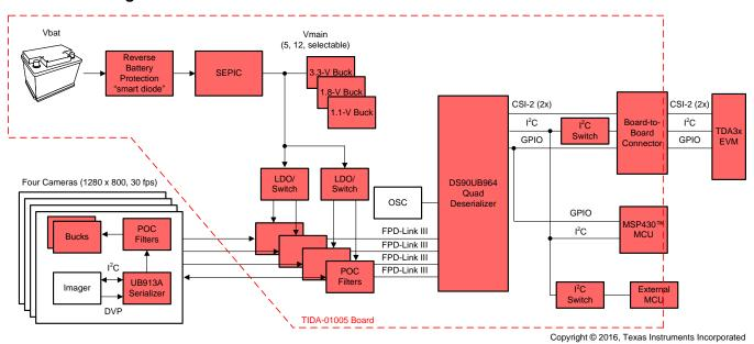
Figure 1. TIDA-01005 Block Diagram and System Partition
