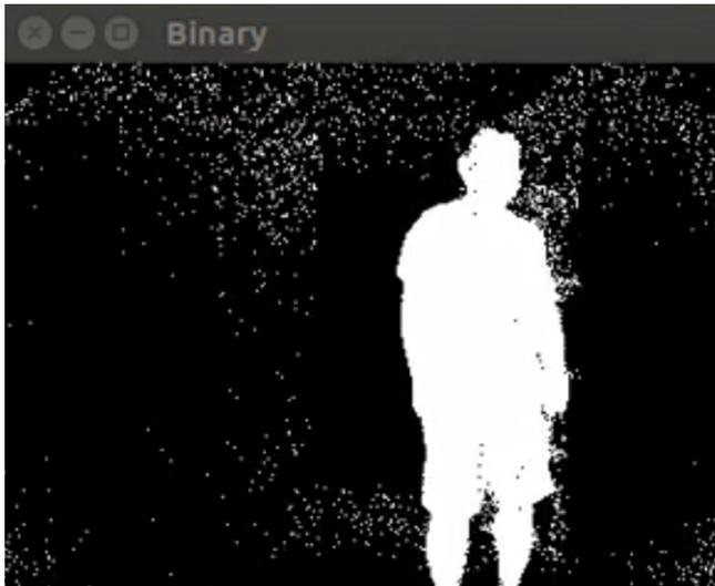
Figure 10. Background Subtraction Binary Image
