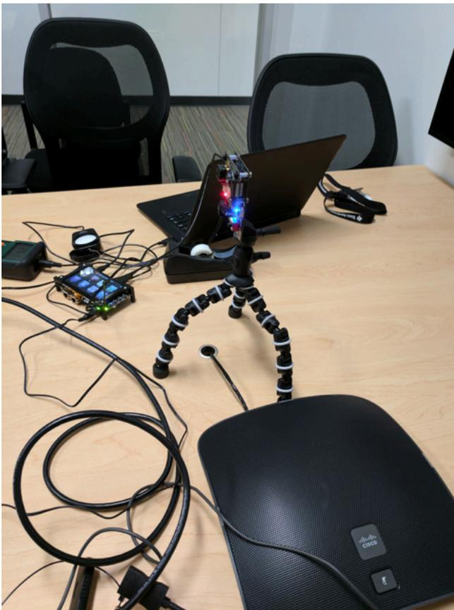
**Figure 23. OPT8241 CDK and AM437x GP EVM With Tripod**
