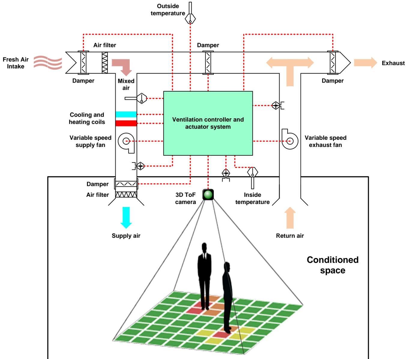
Figure 9. 3D ToF Camera Based DCV System
