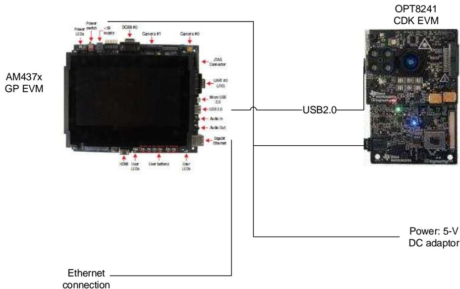
Figure 15. Hardware Setup
