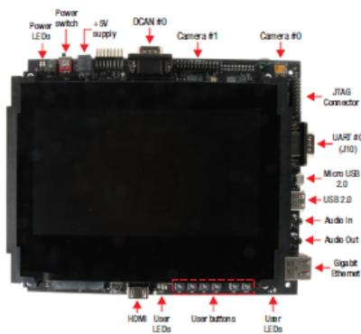
Figure 7. AM437x GP EVM Top View
