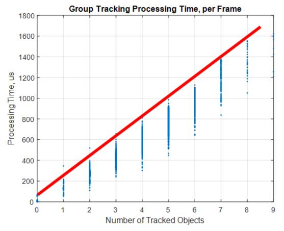
We observed that processing time increases linearly with number of tracking objects. With fixed number of tracking objects, complexity increases linearly with number of input points. Taking the worst case of number of points per frame of 250, we can derive a bound of about  $\approx$  200µs per tracking object. With frame time of 50ms, tracking 20 targets shall be completed in 4ms, which will consume <10% of CPU.
