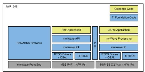
Figure 2. Generic mmWave SDK Software Block Diagram
