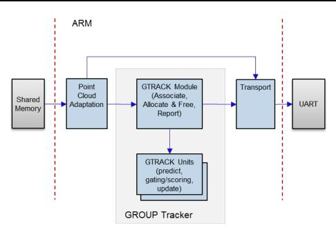
Figure 5. High Level Radar Processing
