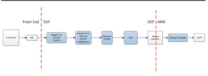
Figure 4. Low Level Radar Processing
