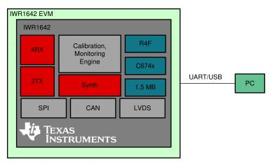
Figure 1. Hardware Block Diagram
