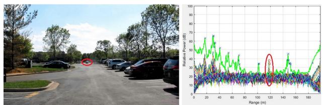
Figure 32. Scenario Three: 120-m Ground Truth (left) and Range Profile (right)
