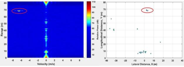
Figure 27. Scenario One: Heatmap Snapshot (left) and X-Y Detections (right)
