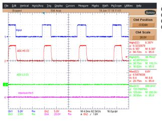
Figure 44. TIDA-01445 Short Circuit to Ground at Pin 1
