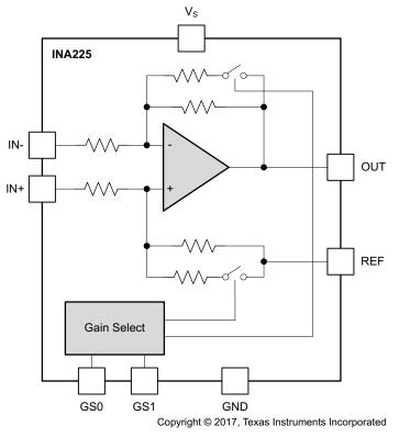
Figure 4. INA225-Q1 Block Diagram
