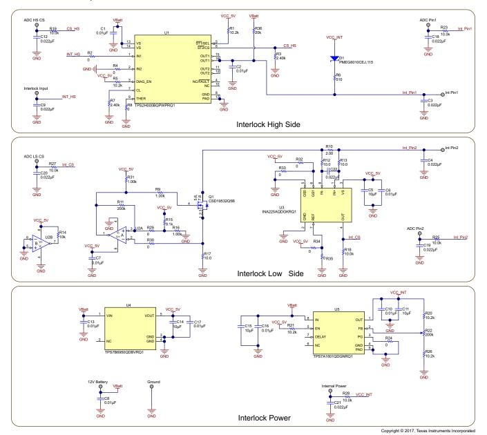
Figure 13. TIDA-01445 Schematic
