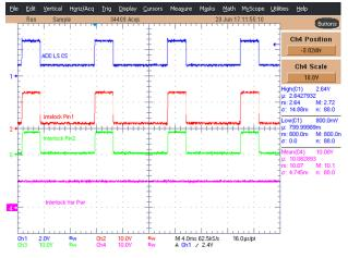
Figure 24. Interlock VCC at 10 V
