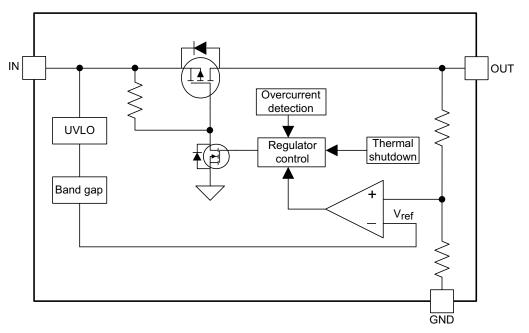
Figure 6. TPS7B6950-Q1 Block Diagram
