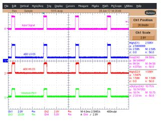
Figure 38. TIDA-01445 for 95 Hz and 10% Duty Cycle
