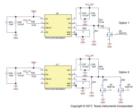
Figure 16. Configurable VCC INT
