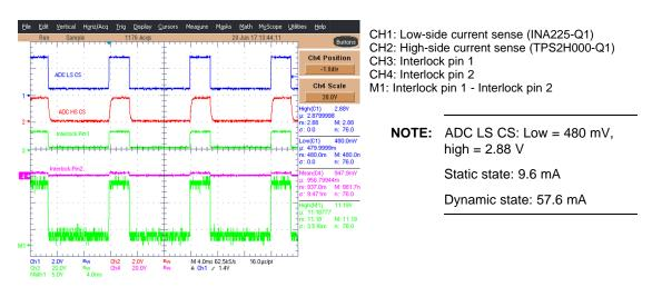
Figure 34. TIDA-01445 at 200- $\Omega$  Load Resistance
