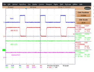
Figure 46. TIDA-01445 Short Circuit to Battery at Pin 1
