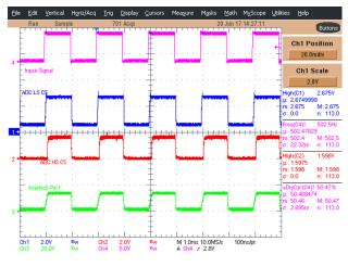
Figure 36. TIDA-01445 for 500 Hz and 50% Duty Cycle
