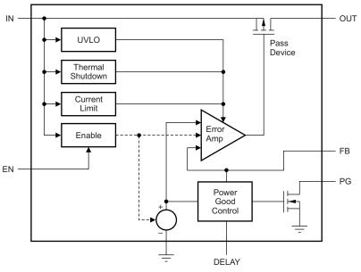
Figure 5. TPS7A1601-Q1 Block Diagram
