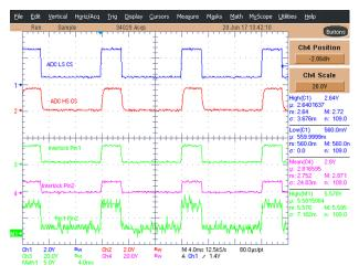
CH1: Low-side current sense (INA225-Q1) CH2: High-side current sense (TPS2H000-Q1) CH3: Interlock pin 1 CH4: Interlock pin 2 M1: Interlock pin 1 - Interlock pin 2
