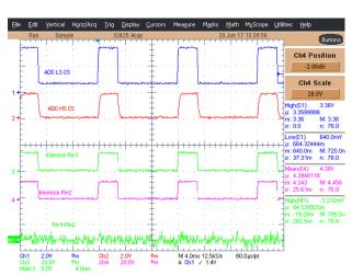
Figure 30. TIDA-01445 at 0-Ω Load Resistance
