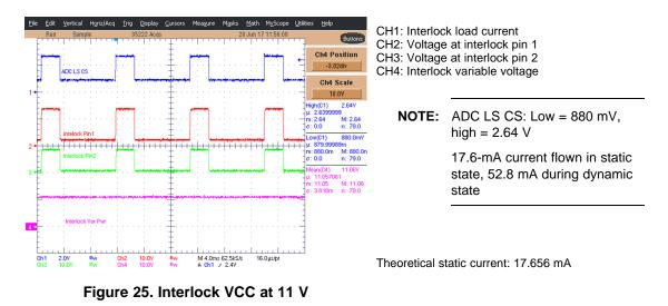
These figures shows an increase in the interlock static current. Based on interlock resistance required by OEM, R6 and VCC INT can be set to get the required static state current.
