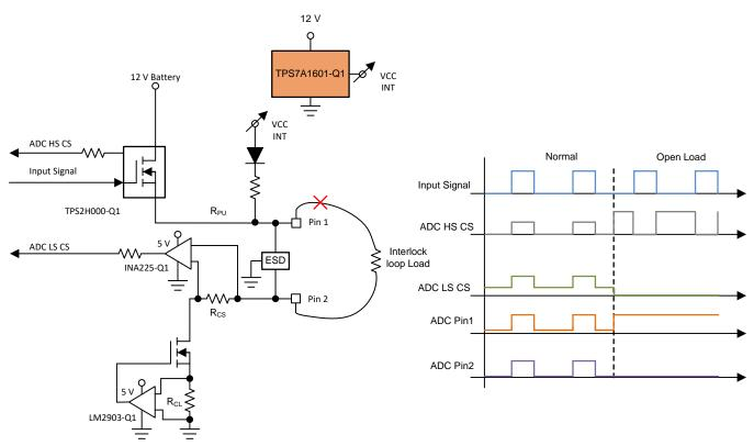
Figure 12. Interlock Line Open Load
