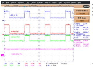
Figure 23. Interlock VCC at 9 V
