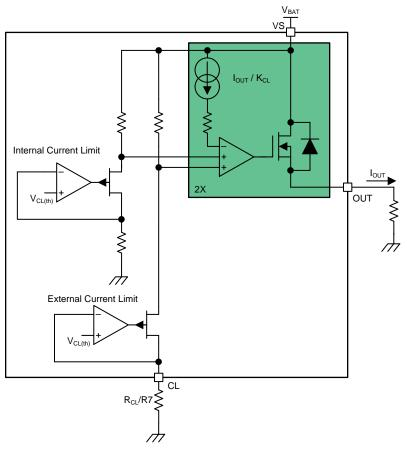
Figure 14. TPS2H000-Q1 Current Limit
