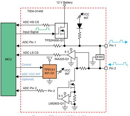
Figure 2. TIDA-01445 Block Diagram
