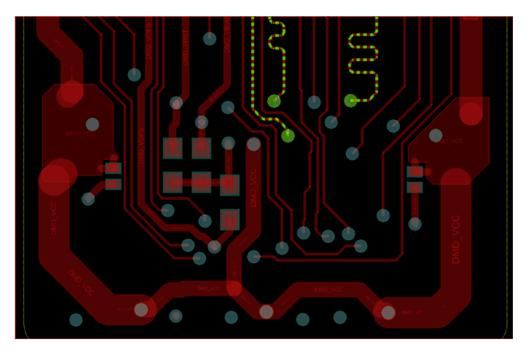
Figure 13. DMD Flex Cable—Bottom Layer
