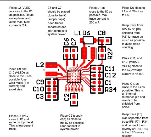
Figure 14. Layout Example for Switching Power Supply
