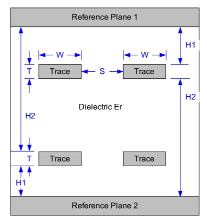
Figure 11. PCB Stacking Geometries
