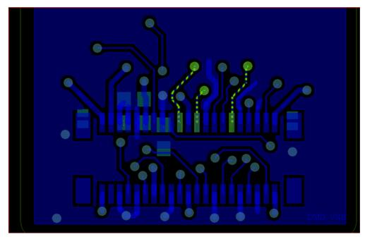
Figure 12. DMD Flex Cable—Top Layer
