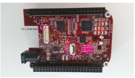
Figure 4. Overview of Board Pinout
