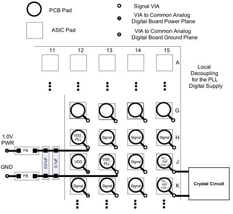
Figure 10. PLL Filter Layout
