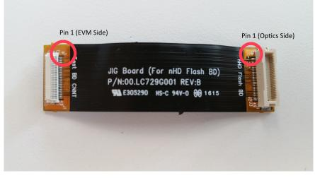
Figure 2. Overview of Flex Cable Pinout for 0.2 nHD Optical Engine
