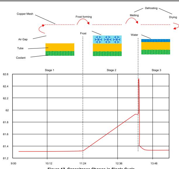
Figure 17. Capacitance Change in Single Cycle
