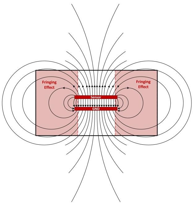
Figure 6. Electric Fields of Parallel Plate Capacitor
