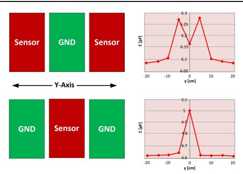
Figure 12. Central Ground, Central Sensor Symmetry
