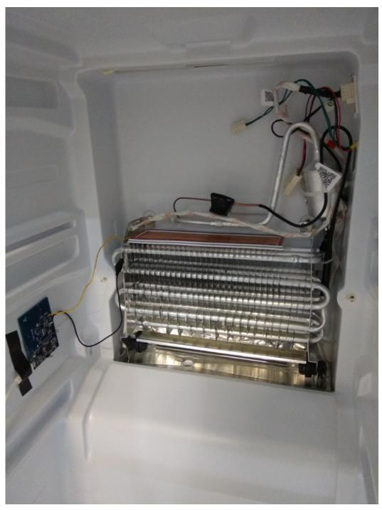
Figure 23. Evaporator In Refrigerator
