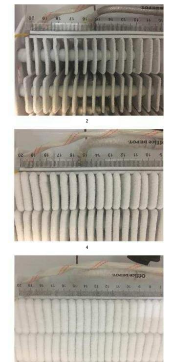
Figure 29. Frost Forming Process
