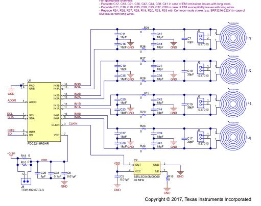
Figure 9. Schematic for Capacitance Detection Circuits
