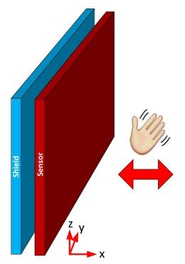
Figure 14. Single-Sensor Topology for Human Recognition
