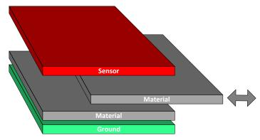
Figure 10. Parallel Plate Topology for Material Analysis
