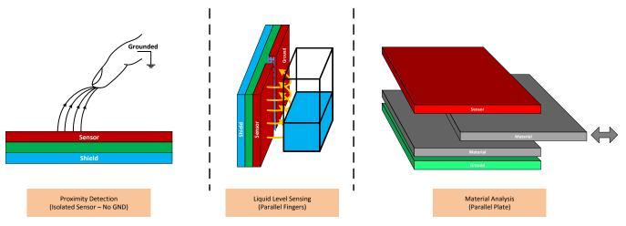
Figure 7. Basic Implements for Capacitive Sensing
