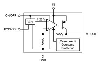
Figure 3. LP2985-N Functional Block Diagram
