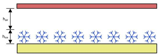
Figure 8. Model for Frost and Ice Detection Based on Capacitance
