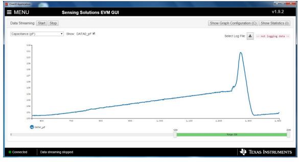
Figure 36. Capacitance Curve in Single Cycle
