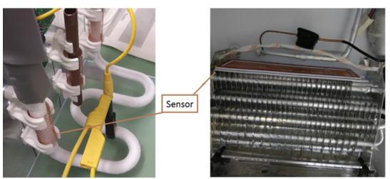
Figure 16. Capacitive Sensor
