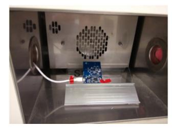
Figure 31. Temperature Drift Test Setup
