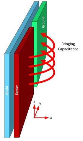
Figure 11. Parallel Fingers (GND Sensor) Topology
