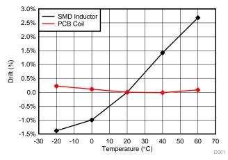
Figure 32. Capacitance Temperature Drift For PCB Coil and Common SMD Inductor
