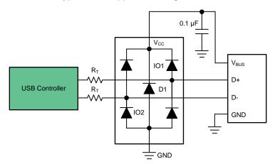
Figure 4. TPD2E001 Typical USB Application Diagram
