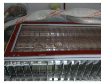
Figure 34. Waterdrop on Surface of Sensor
