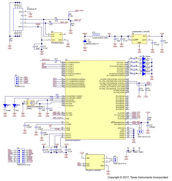
Figure 21. Schematic for Auxiliary Control Board
