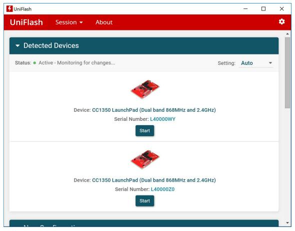
Figure 5. UniFlash v4.2 With Two CC1350LP Boards (for Meter and Data Collector)
