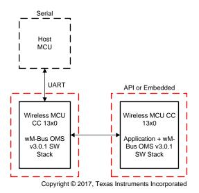
Figure 3. Two TI wM-Bus Stack Alternatives (Serial and Embedded or API)
