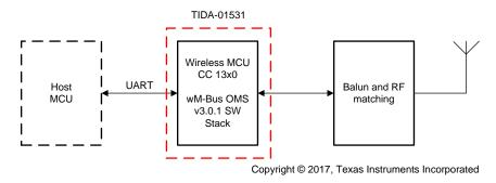
Figure 1. TIDA-01531 Block Diagram
