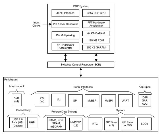
Figure 2. TMS320C5517 DSP Block Diagram
