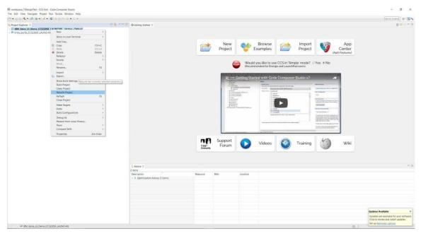
Figure 17. Rebuild CCS Project
