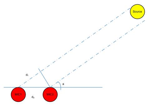
Figure 4. Differences in Distance, Time, and Phase Between Two Microphones
