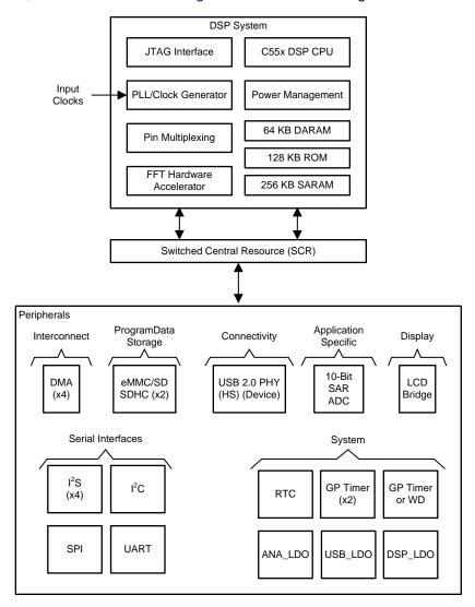
Figure 3. TMS320C5545 Block Diagram
