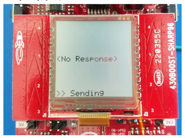
Figure 46. Sharp <sup>®</sup> LCD Indicates Sending Audio to IBM Watson <sup>®</sup> Servers in Progress
