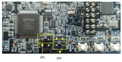
Figure 12. BOOST5545ULP UART Jumper Details
