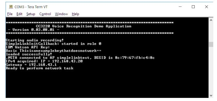
Figure 33. CC3220SF-LAUNCHXL Terminal Emulation Debug Information
