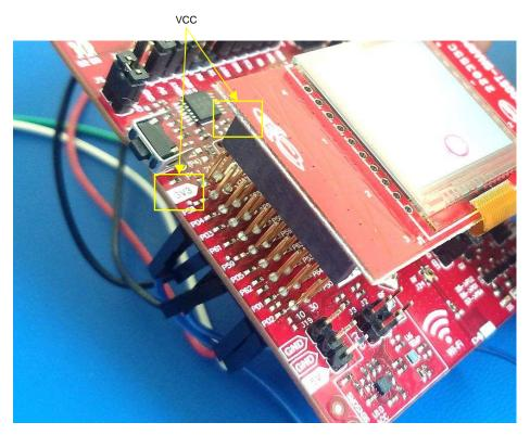
Figure 9. Connecting CC3220SF-LAUNCHXL to 430BOOST-SHARP96
