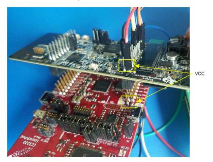
Figure 13. Connecting CC3220SF-LAUNCHXL to BOOST5545ULP
