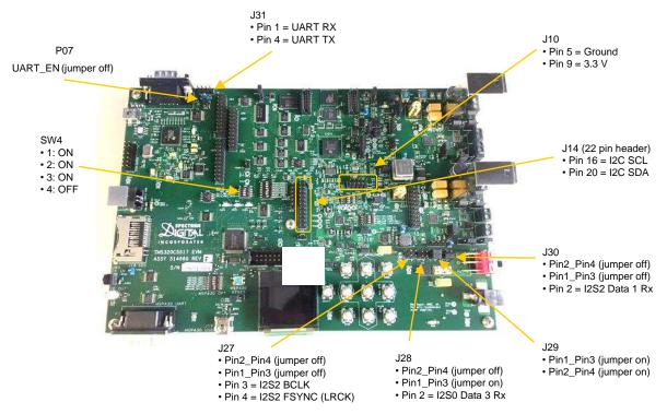
Figure 8. EVM5517 and LMB Wiring Illustration
