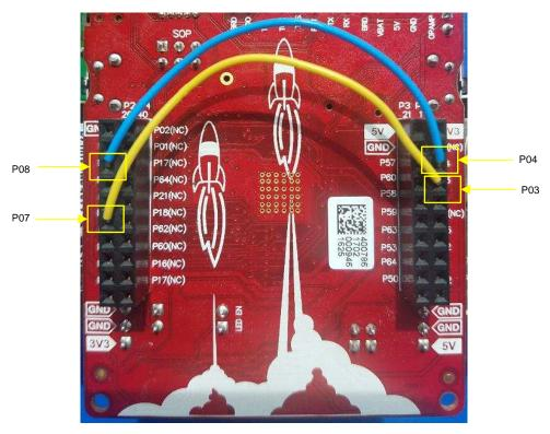
Figure 15. Jumper Wires Required on CC3220SF-LAUNCHXL
