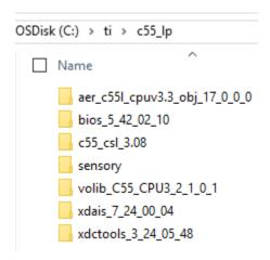
Figure 42. Directory Structure of Project Dependencies and CSL Installation on PC
