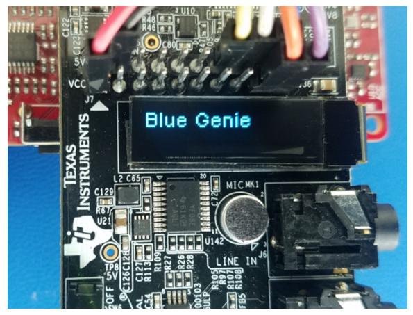
Figure 52. BOOST5545ULP OLED Shows Trigger Phrase After Positive Recognition
