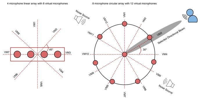
Figure 41. Description of Virtual Microphone
