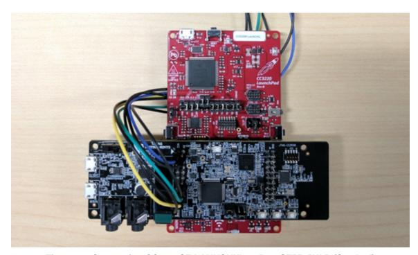
Figure 14. Connecting CC3220SF-LAUNCHXL to BOOST5545ULP (Stacked)
