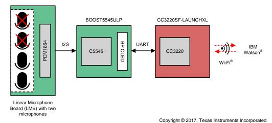
Figure 11. C5545-Based Voice Transcription Demonstration Block Diagram
