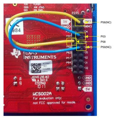
Figure 10. Jumper Wires Required on CC3220SF-LAUNCHXL
