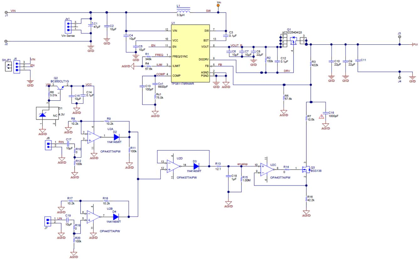
**Figure 2.1 Schematic of the PMP15036 (Boost Converter)**
