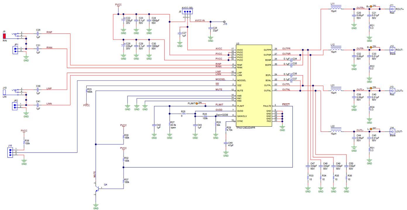
**Figure 2.2 Schematic of the PMP15036 (Power Amplifier)**
