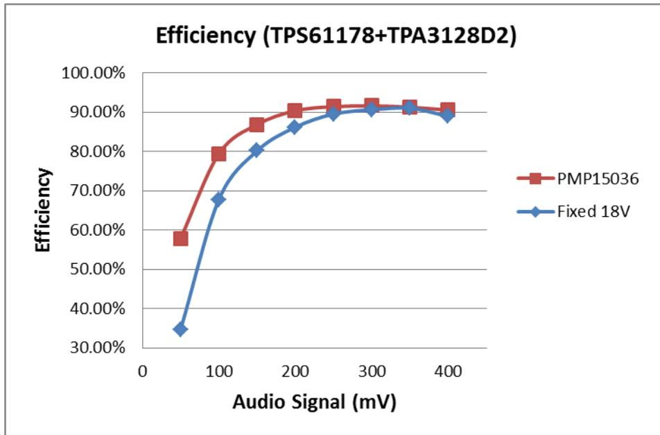
Figure 6 Efficiency Comparison Result ( $V_{in}=7.2V$ ,  $R_o=4\text{ ohm}$ )
