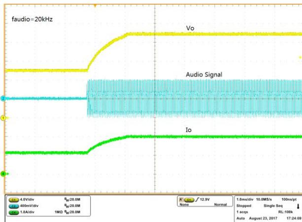
Figure 4.1 Output Voltage Transition at  $f_{audio}=20\text{kHz}$
