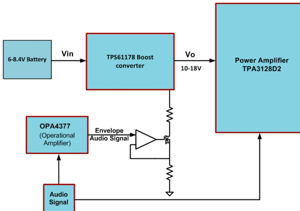
Figure 1. Block Diagram of the PMP15036
