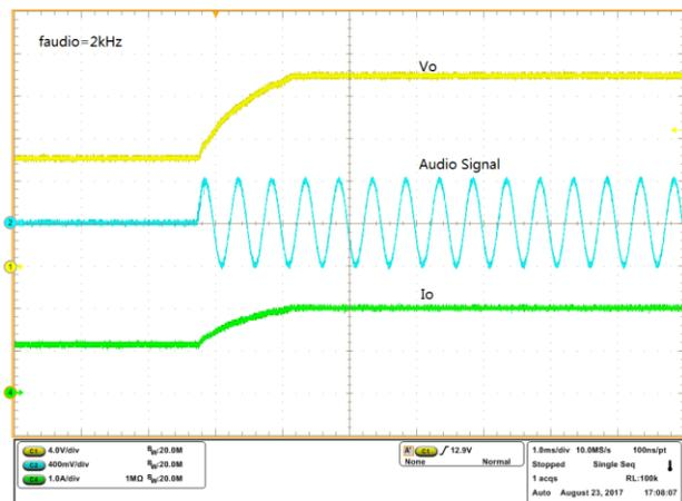
Figure 4.2 Output Voltage Transition at  $f_{audio}=2\text{kHz}$
