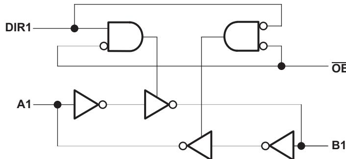
**Figure 5. SN74AVC4T774 Functional Block Diagram**
