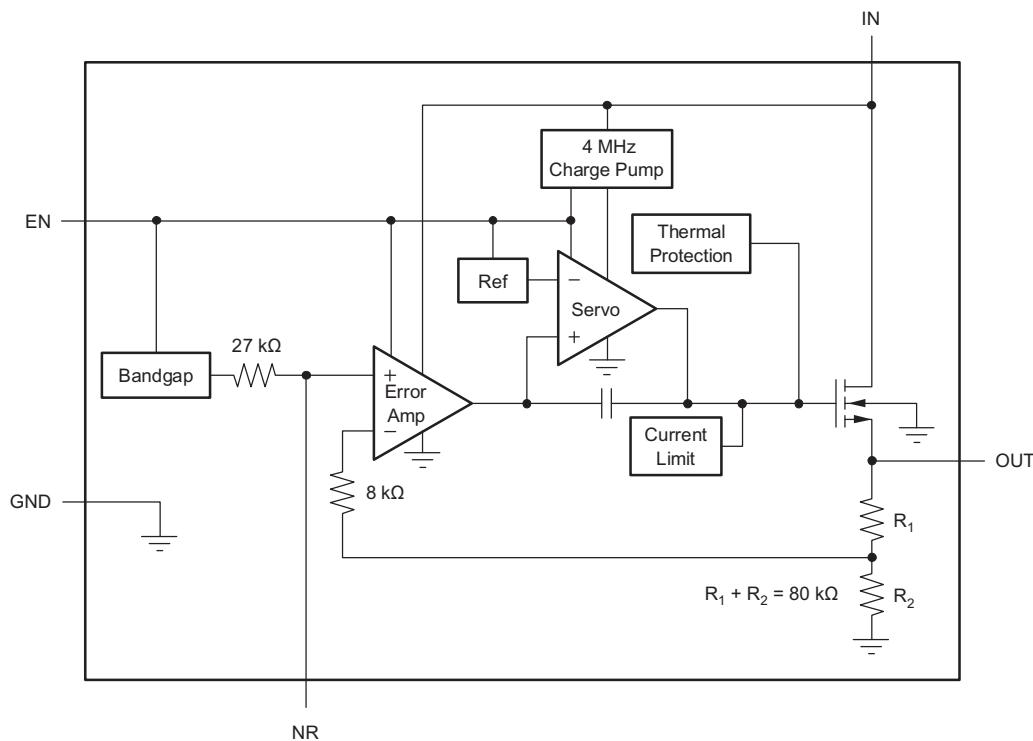
**Figure 6. TPS736xx Functional Block Diagram**
