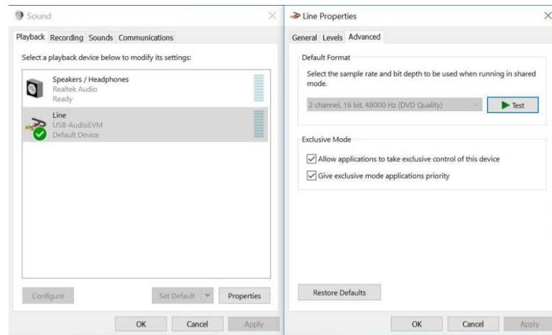
**Figure 13. Desired Microsoft® Windows® Sound Card Settings for Reference Design Board**
