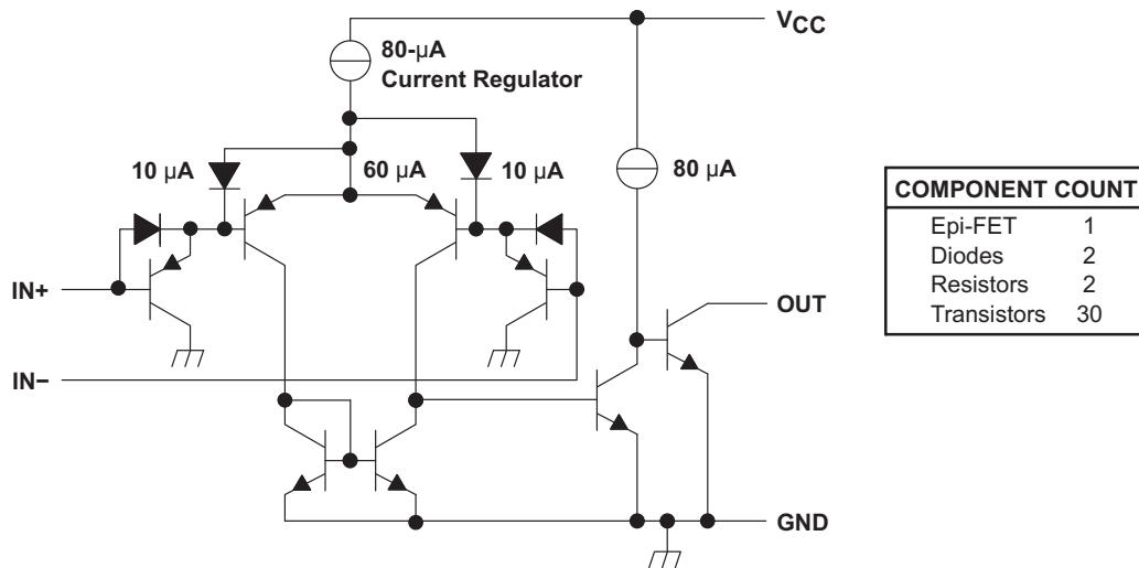
Figure 7. LM2903-Q1 Block Diagram
