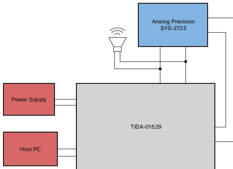
**Figure 17. Test Setup Block Diagram for Power Output, THD, and ICN Tests**
