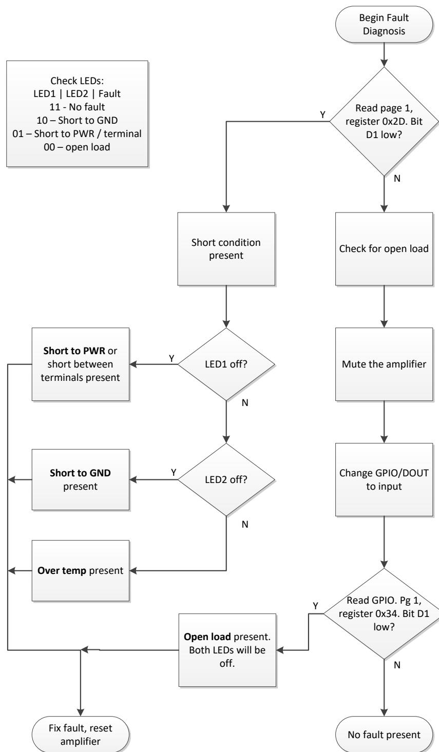
Figure 15. Process for Fault Diagnosis with Diagnostic Circuit #1
