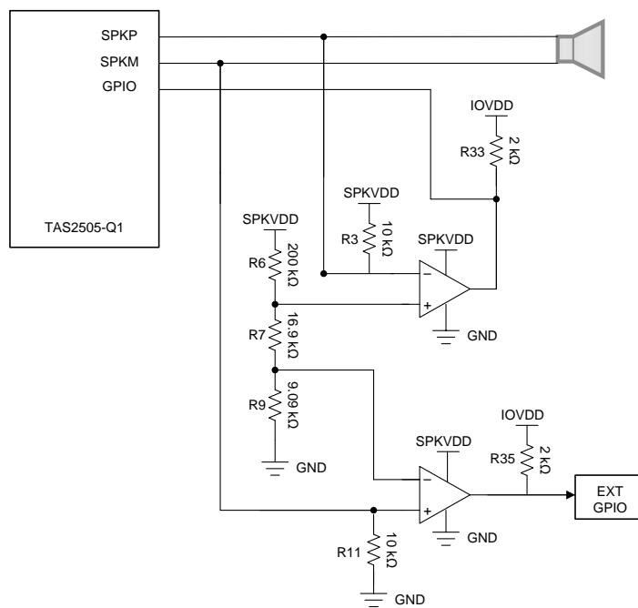
**Figure 10. Diagnostic Circuit #1 Schematic**
