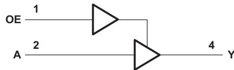
**Figure 4. SN74LVC1G126 Functional Block Diagram**
