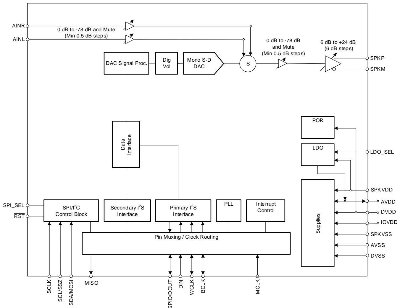
Figure 2. TAS2505-Q1 Functional Block Diagram
