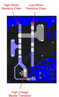
Figure 50. Component Placement of Active Start-Up Circuit
