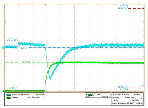
Figure 17. VCC\_8A Load Step Test
