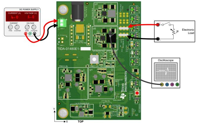
Figure 11. Setup for Measuring Output Voltages with Load Applied
