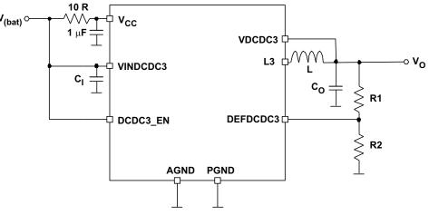
Figure 9. TPS65023 External Resistor Divider for DCDC3
