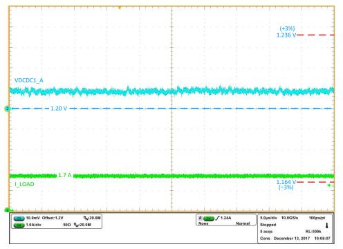
Figure 13. VDCDC1\_A Full Load Test
