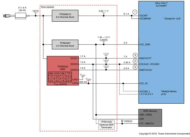
Figure 1. Block Diagram of Design Variant 006
