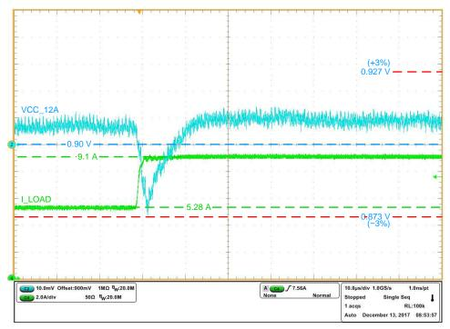
Figure 20. VCC\_12A Load Step Test
