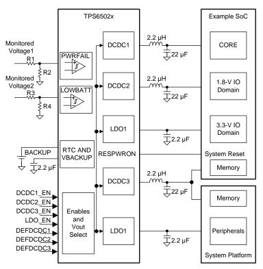
Figure 5. TPS65023 Simplified Application Circuit
