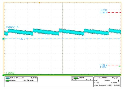
Figure 12. VDCDC1\_A No Load Test
