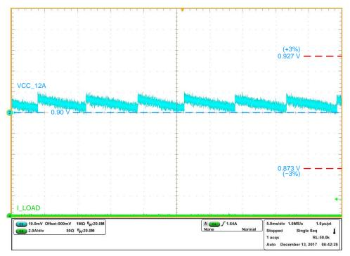
Figure 18. VCC\_12A No Load Test
