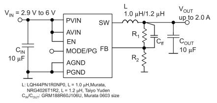
Figure 7. TPS62067 Simplified Application Circuit
