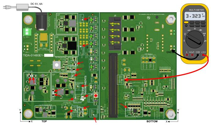
Figure 10. Setup and Measurement Locations for DC Voltage Measurements
