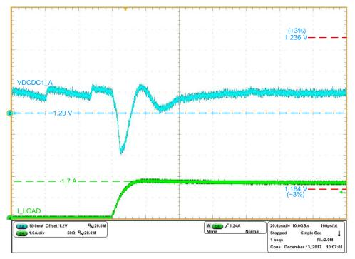
Figure 14. VDCDC1\_A Load Step Test
