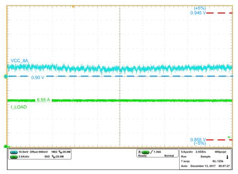
Figure 16. VCC\_8A Full Load Test
