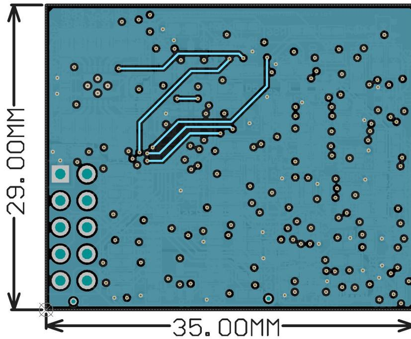
Figure 86. Power Plane of the Reference Design Board
