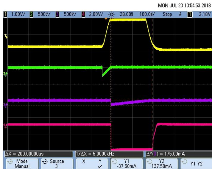
Figure 67. Pacemaker Detection Output (Pulse Duration  $T_D$ ) for 16-mV, 200- $\mu$ s Pace Pulse
