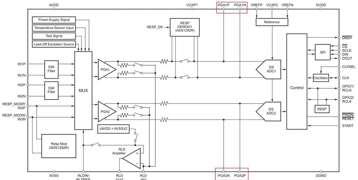
Figure 9. ADS129X Functional Block Diagram
