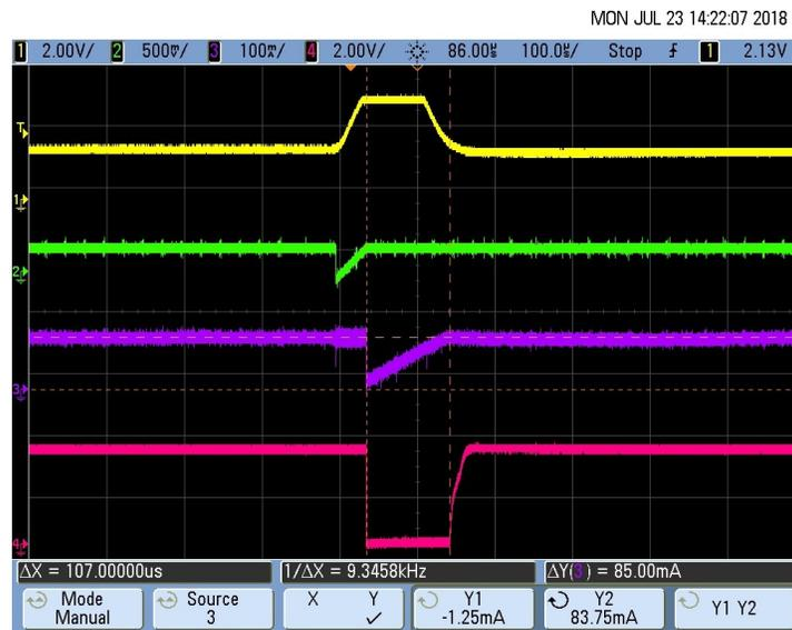
Figure 65. Pacemaker Detection Output (Pulse Duration  $T_D$ ) for 16-mV, 100- $\mu$ s Pace Pulse
