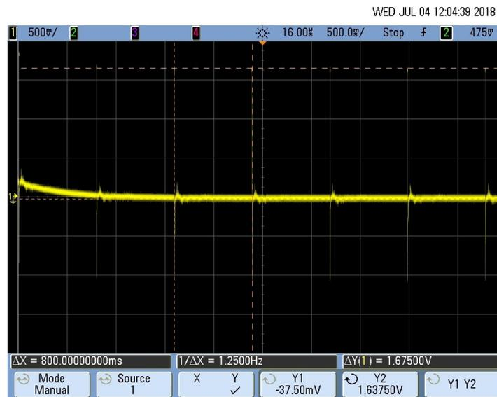
Figure 39. 16-mV Pace Signal 5 at the Output of the Gain Stage Interface With ADS1292
