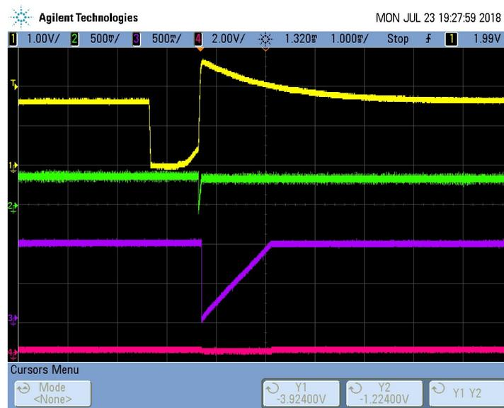
Figure 81. Negative Pace Signal Detection - Negative Pace Pulse Undetected
