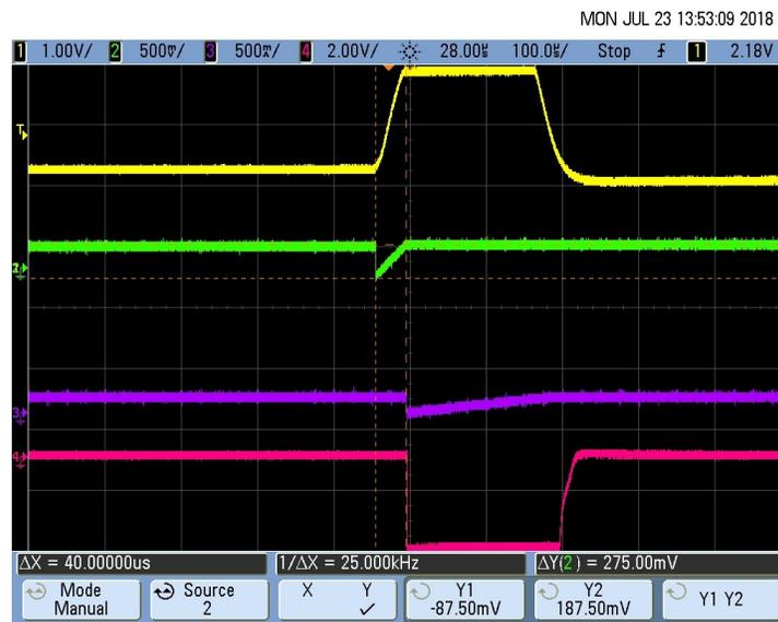
Figure 66. Pacemaker Detection Output (Rise Time  $T_R$ ) for 16-mV, 200- $\mu$ s Pace Pulse
