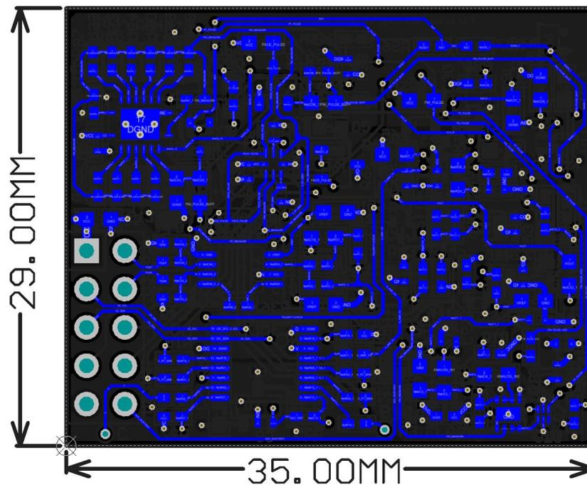
Figure 88. Bottom Layer of the Reference Board
