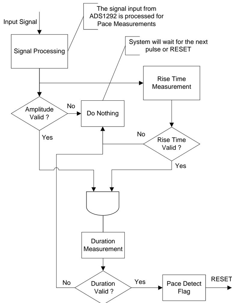
Figure 7. TIDA-010005 System Flow Diagram
