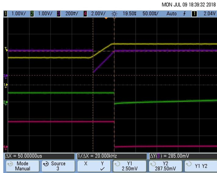
Figure 44. Rise Time Measurement of the Pace Signal ( $T_R = 50 \mu\text{s}$ )
