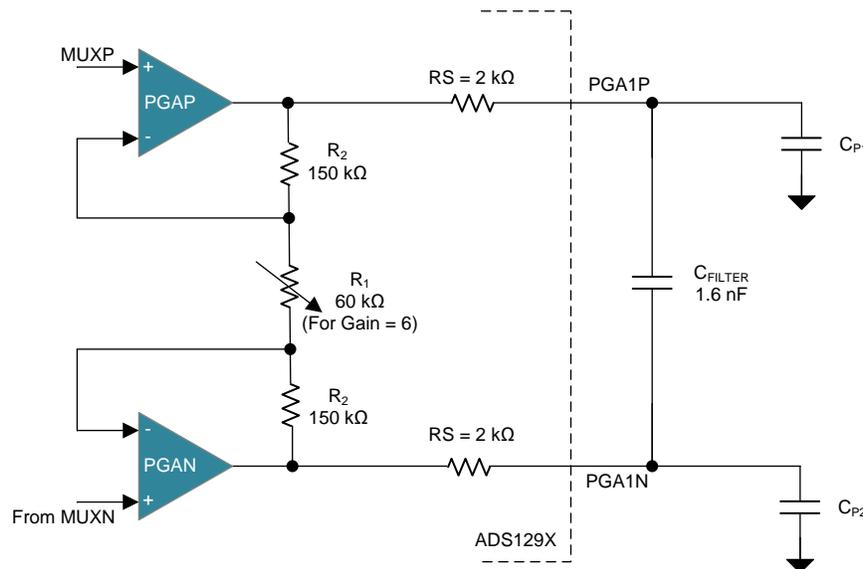
Figure 10. PGA Implementation in ADS129X Device
