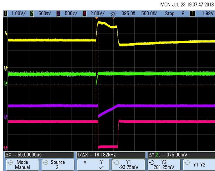
Figure 60. Pacemaker Detection Output (Rise Time  $T_R$ ) for 8-mV, 500- $\mu$ s Pace Pulse
