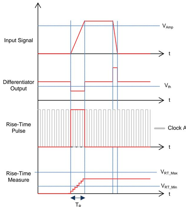
**Figure 5. Rise Time Pulse Generation and Measurement**
