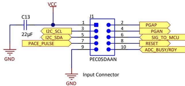
**Figure 8. Input Connector to TIDA-010005**
