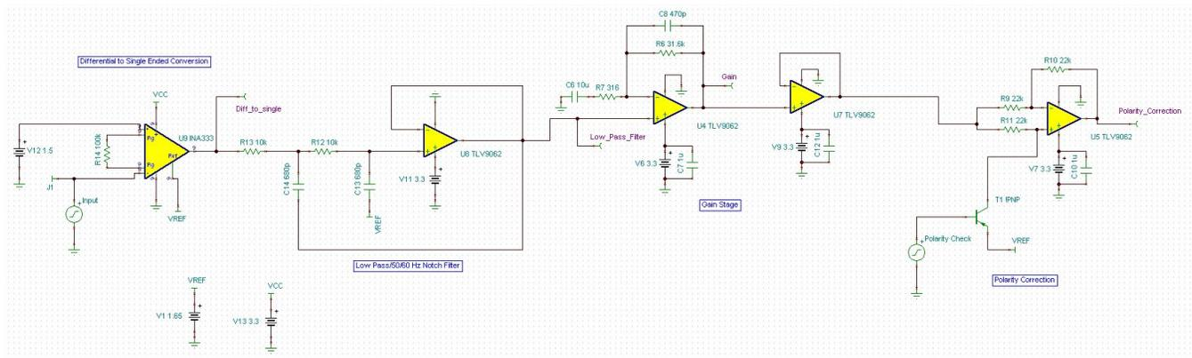
Figure 24. TINA-TI™ Schematic of the Entire Signal Processing Section
