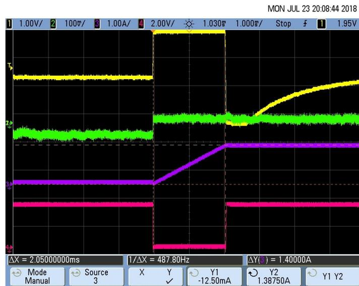
Figure 80. Pacemaker Detection Output (Pulse Duration  $T_D$ ) for 700-mV, 2-ms Pace Pulse
