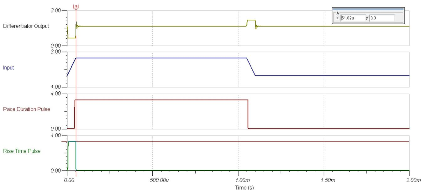
Figure 29. Simulation Output of the Signal Measurement Section Till TTL Pulse Generation
