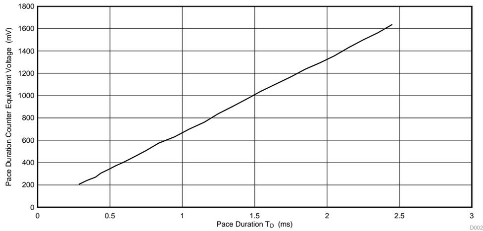
Figure 52. Equivalent Analog Voltage of the Pulse Duration Counter (mV) vs the Pulse Duration  $T_D$  (ms)
