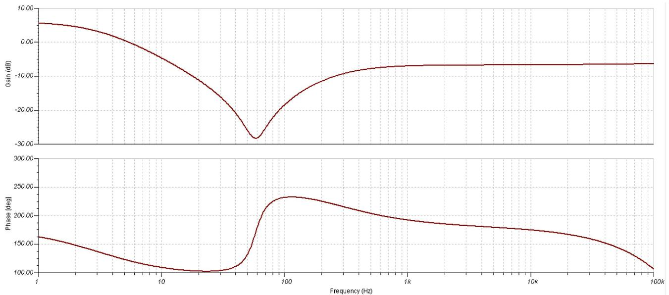
Figure 17. Frequency and Phase Response of the 60-Hz Notch Filter From 1 Hz to 100 kHz
