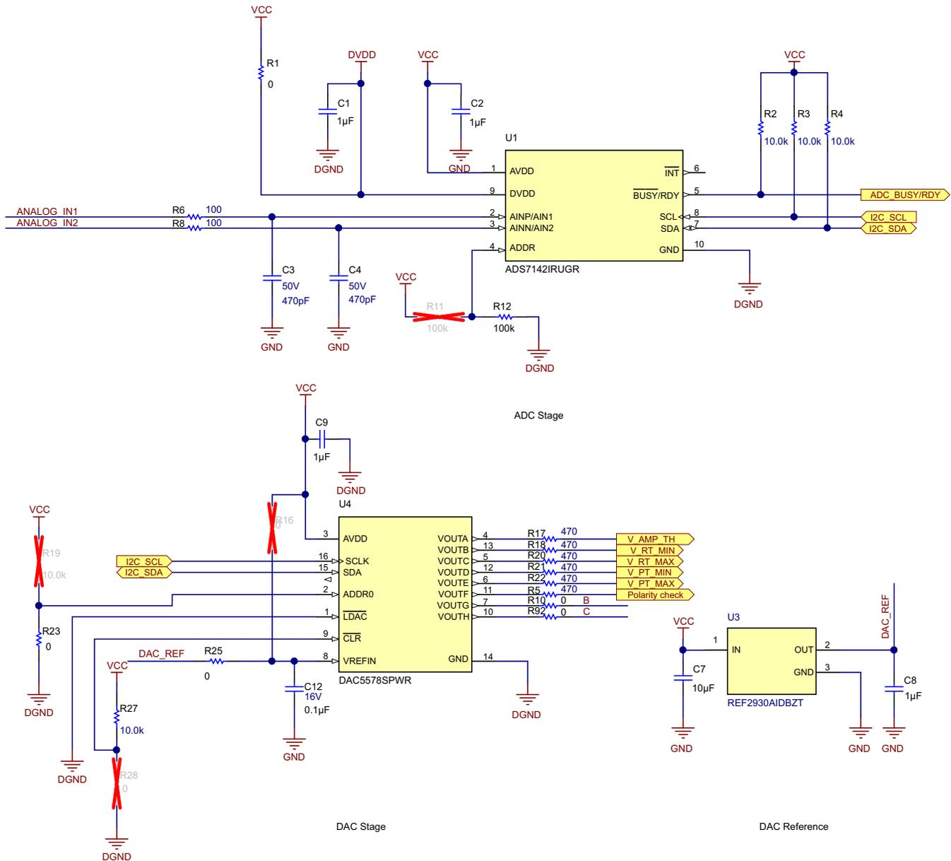
Figure 31. ADC & DAC Implementation in the Reference Design
