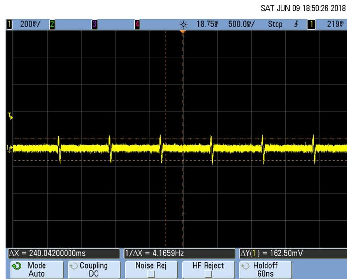
Figure 38. 5 mV ECG Signal at the Output of the Gain Stage Interfaced With ADS1292
