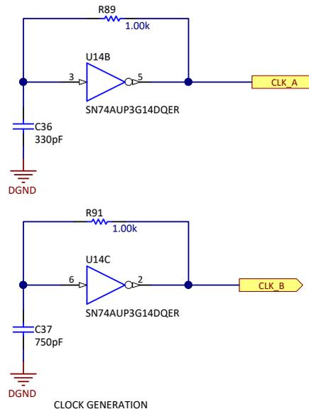
**Figure 30. Circuitry Implemented to Generate Onboard Counter Clocks**
