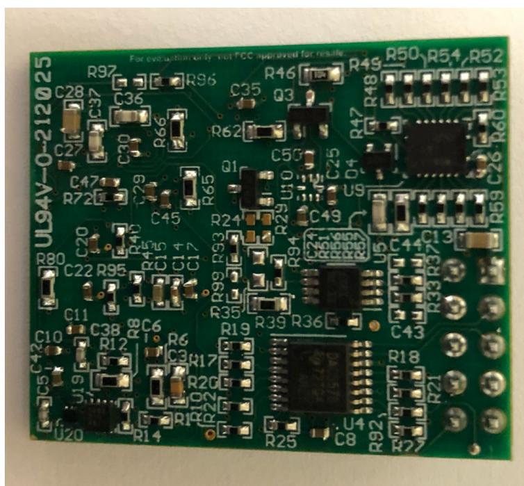
Figure 33. Reference Design PCB (Bottom View)
