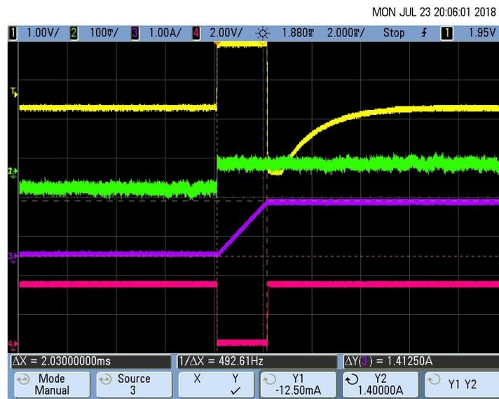
Figure 78. Pacemaker Detection Output (Pulse Duration  $T_D$ ) for 500-mV, 2-ms Pace Pulse
