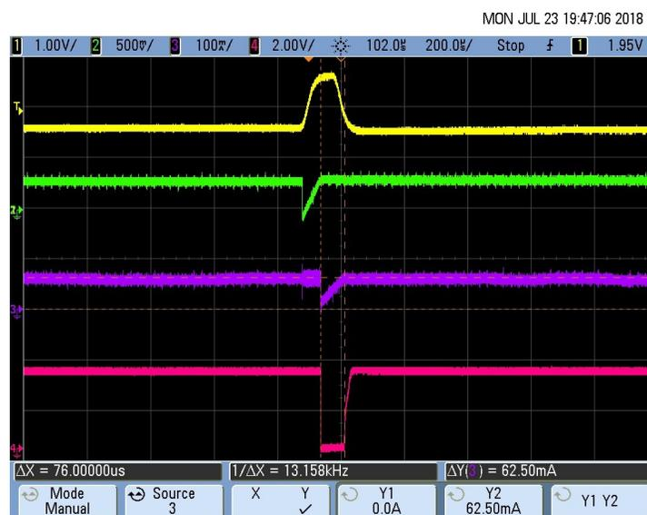
Figure 57. Pacemaker Detection Output (Pulse Duration  $T_D$ ) for 8-mV, 100- $\mu$ s Pace Pulse
