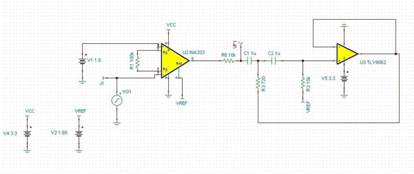
Figure 18. TINA-TI™ Simulation Circuit of the 50-Hz Notch Filter
