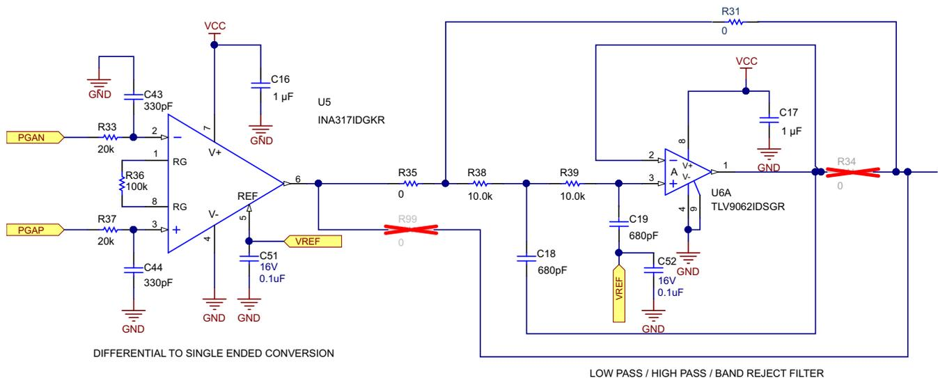
Figure 15. 50, 60 Hz Notch Filter Schematics for the Filter Implementation
