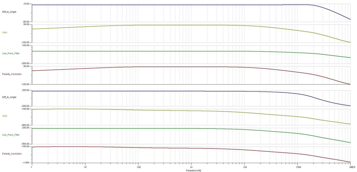
Figure 26. Magnitude and Phase Response of the Entire Signal Processing Section From 1 Hz to 1 MHz
