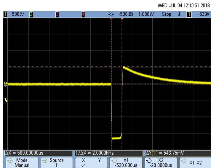
Figure 41. Negative Pace Signal From the Patient Simulator Interfaced With ADS1292
