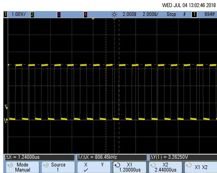
Figure 54. Clock (CLK B) Input to the Pulse Duration Counter
