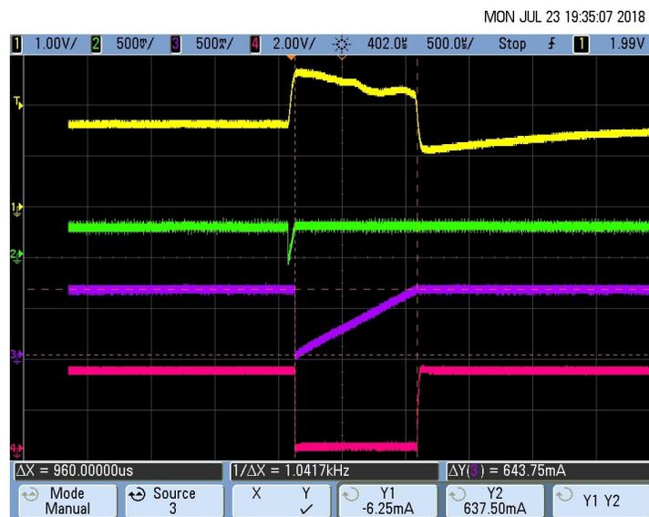
Figure 63. Pacemaker Detection Output (Pulse Duration  $T_D$ ) for 8-mV, 1-ms Pace Pulse
