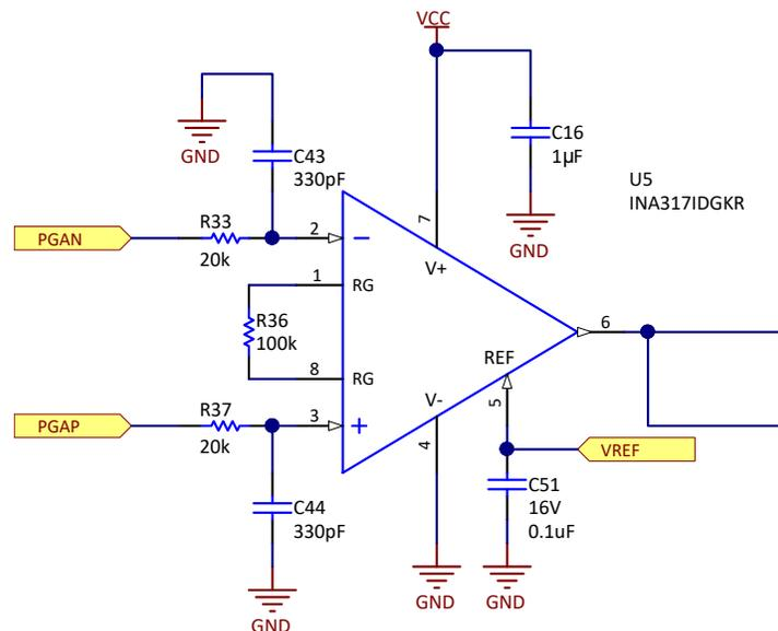
Figure 11. Differential to Single-Ended Conversion Circuit
