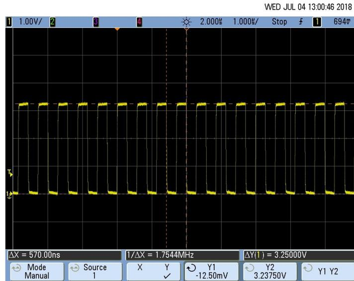
Figure 53. Clock (CLK A) Input to Rise Time Counter
