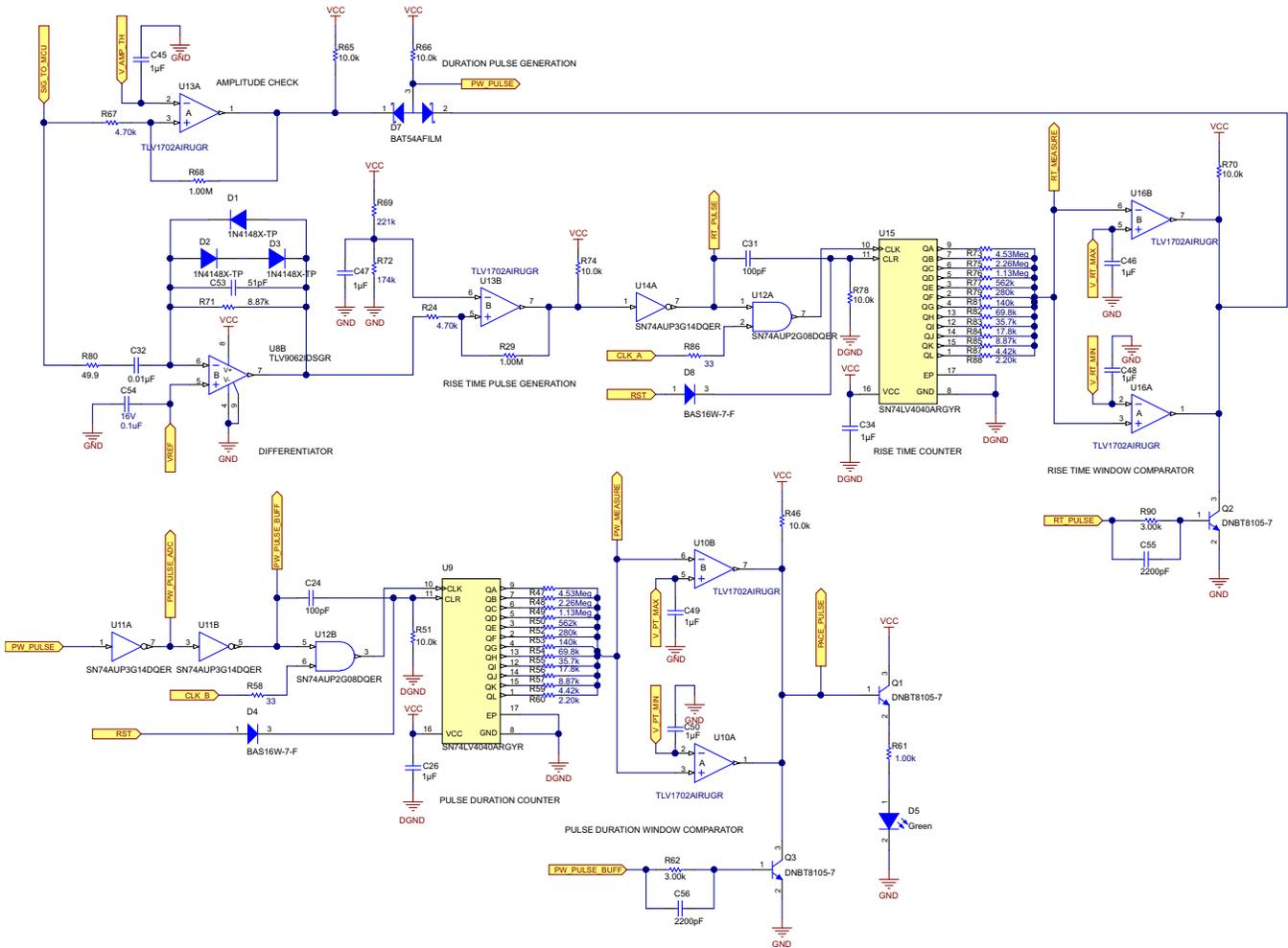
Figure 27. Signal Measurement Section Schematic
