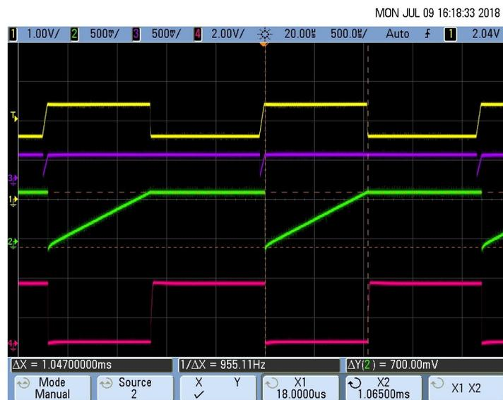
Figure 55. Pacemaker Detection Output for 8-mV, 100-μs Pace Pulse
