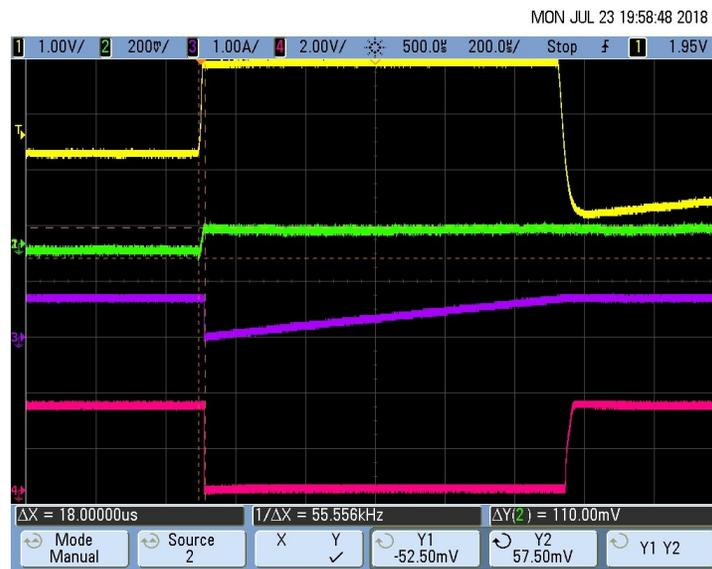
Figure 74. Pacemaker Detection Output (Rise Time  $T_R$ ) for 50-mV, 1-ms Pace Pulse
