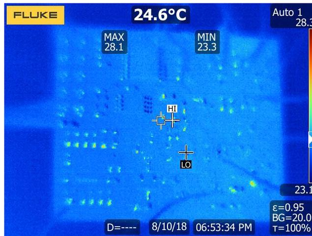
Figure 84. Thermal Image of the Bottom Section of TIDA-010005
