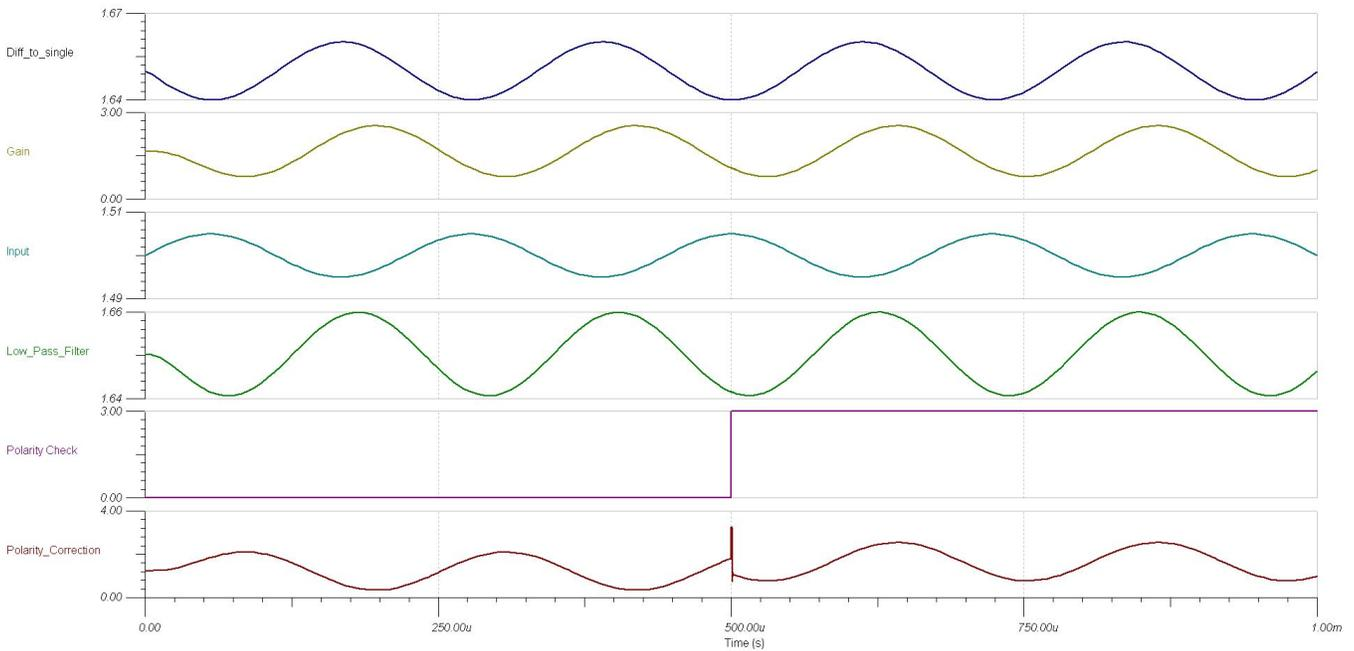
Figure 25. TINA-TI™ Simulation Output Characteristics of Entire Signal Processing Section
