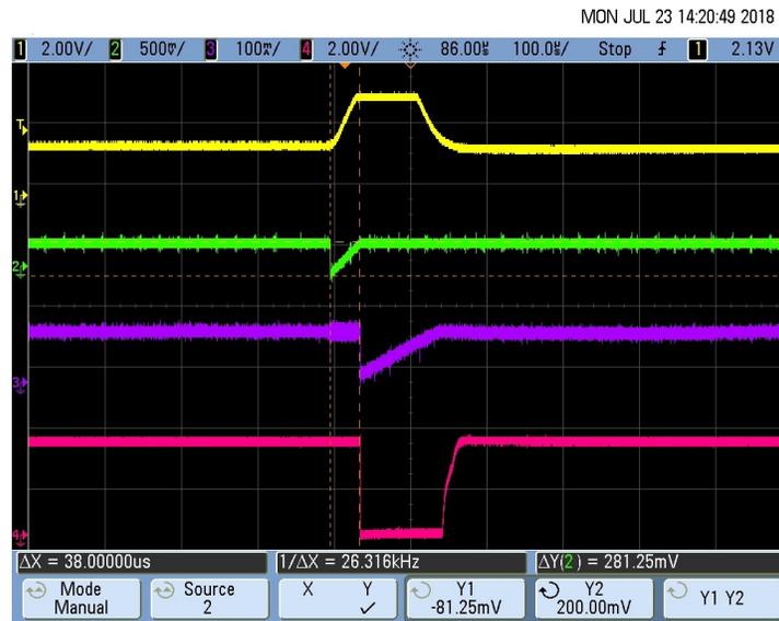
Figure 64. Pacemaker Detection Output (Rise Time  $T_R$ ) for 16-mV, 100- $\mu$ s Pace Pulse
