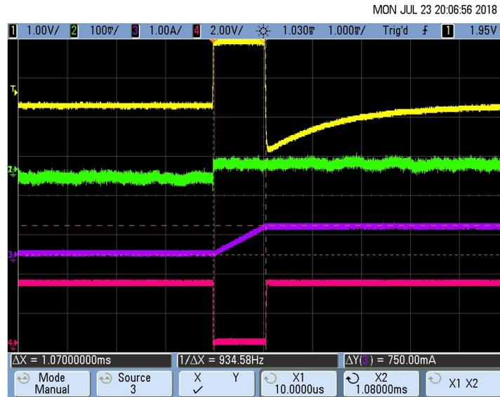
Figure 77. Pacemaker Detection Output (Pulse Duration  $T_D$ ) for 500-mV, 1-ms Pace Pulse
