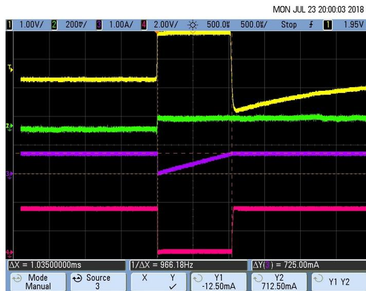
Figure 75. Pacemaker Detection Output (Pulse Duration  $T_D$ ) for 50-mV, 1-ms Pace Pulse
