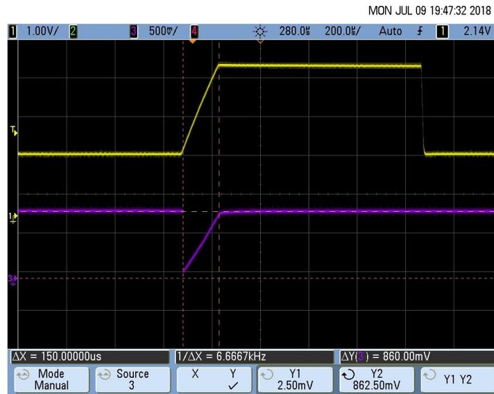
Figure 42. Rise Time Measurement of the Pace Signal ( $T_R = 150 \mu s$ )
