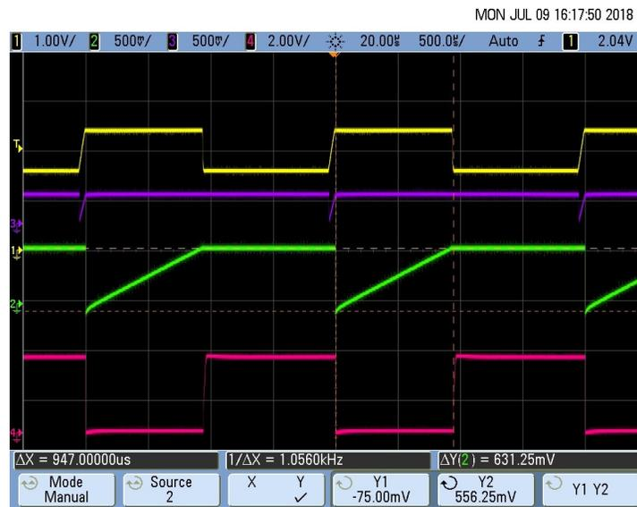
Figure 49. Pulse Duration Measurement of the Pace Pulse ( $T_D = 1 \text{ ms}$ )
