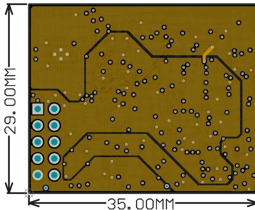
**Figure 85. Ground Planes of the Reference Design Board**
