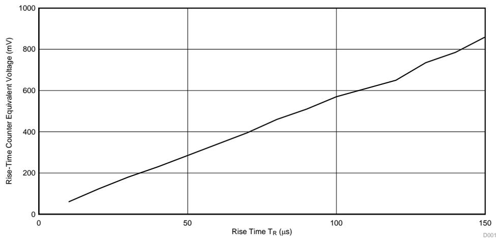
**Figure 47. Equivalent Analog Voltage of the Rise Time Counter (mV) vs the Rise Time  $T_R$  ( $\mu s$ )**
