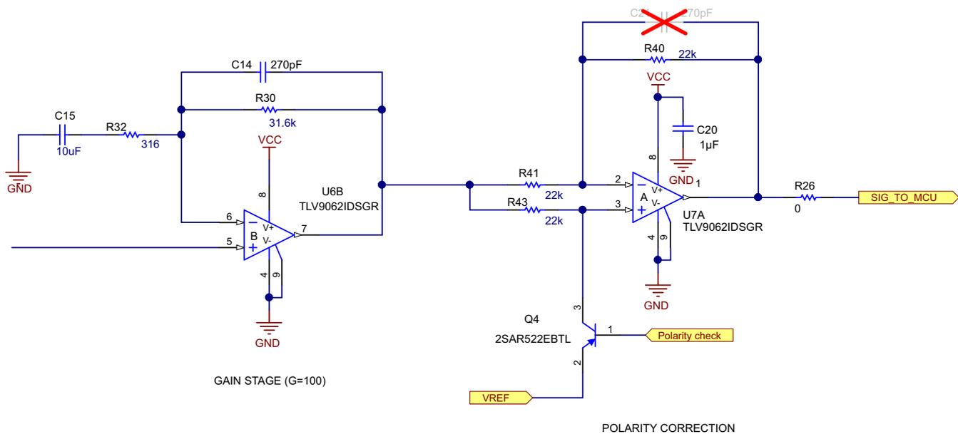
**Figure 20. Gain and Polarity Correction Circuitry Schematic**
