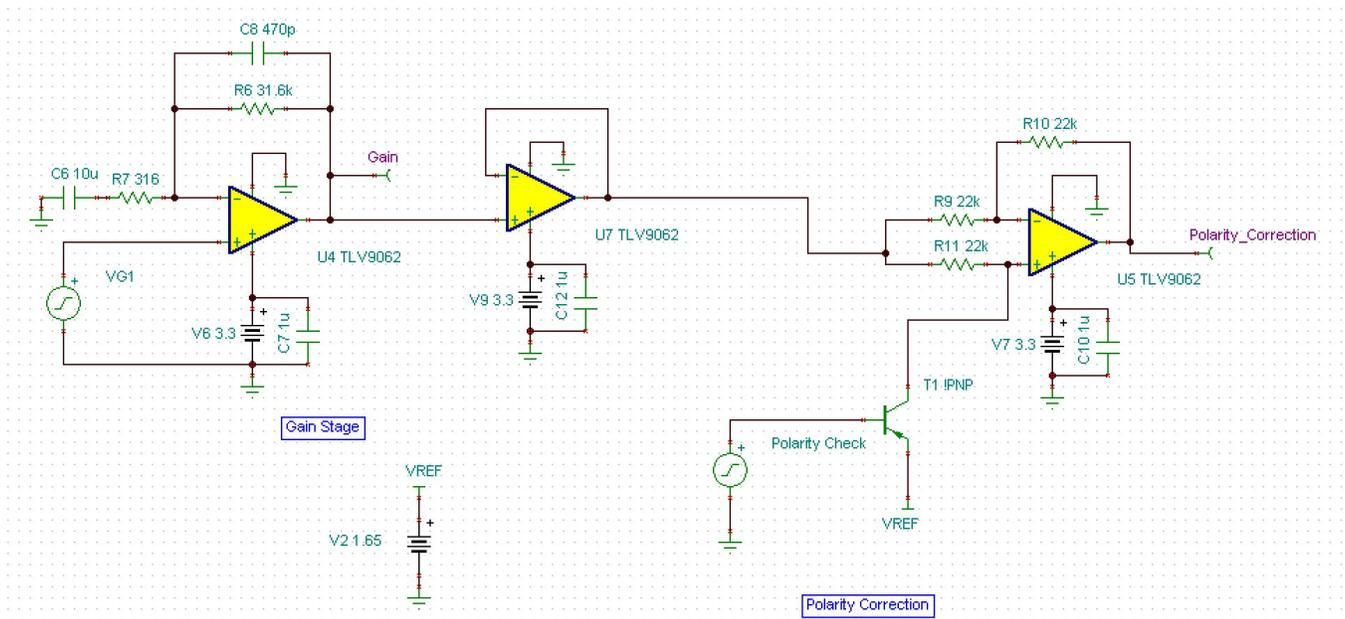
Figure 22. TINA-TI™ Simulation Schematic Gain and Polarity Correction Circuit
