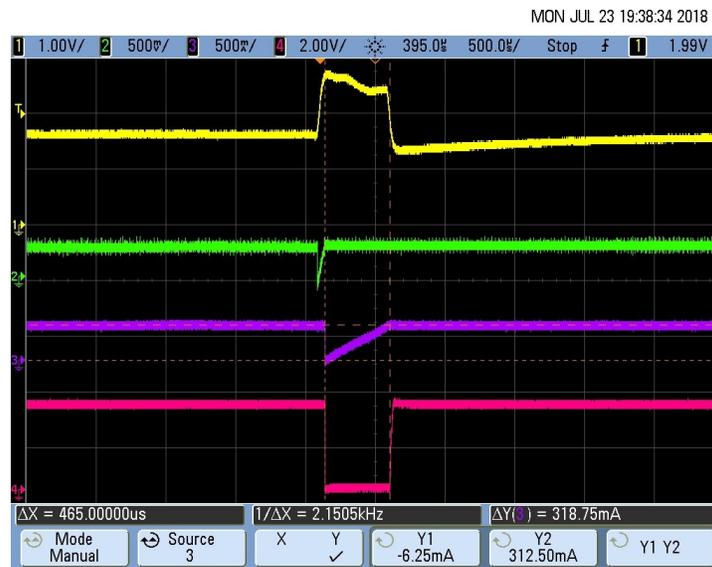
Figure 61. Pacemaker Detection Output (Pulse Duration  $T_D$ ) for 8-mV, 500- $\mu$ s Pace Pulse
