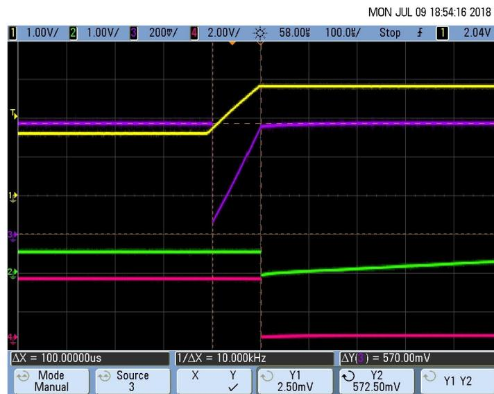
Figure 43. Rise Time Measurement of the Pace Signal ( $T_R = 100 \mu s$ )
