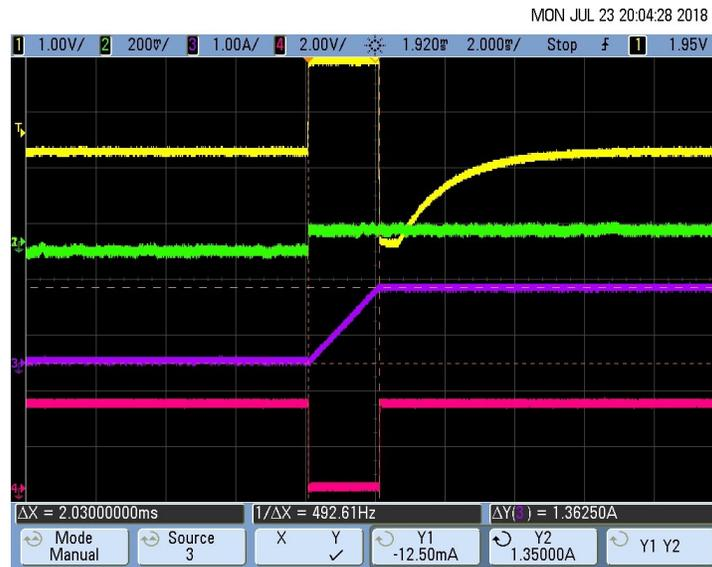
Figure 76. Pacemaker Detection Output (Pulse Duration  $T_D$ ) for 50-mV, 2-ms Pace Pulse
