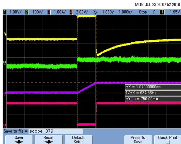
Figure 79. Pacemaker Detection Output (Pulse Duration  $T_D$ ) for 700-mV, 1-ms Pace Pulse
