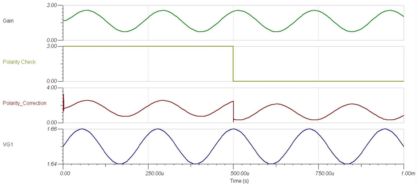
Figure 23. TINA-TI™ Simulation Output Characteristics of Gain and Polarity Correction Circuit
