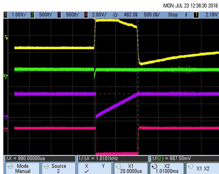
**Figure 71. Pacemaker Detection Output (Pulse Duration  $T_D$ ) for 16-mV, 1-ms Pace Pulse**
