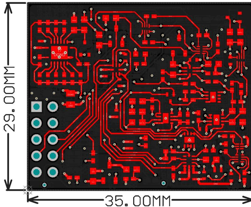
Figure 87. Top Layer of the Reference Board
