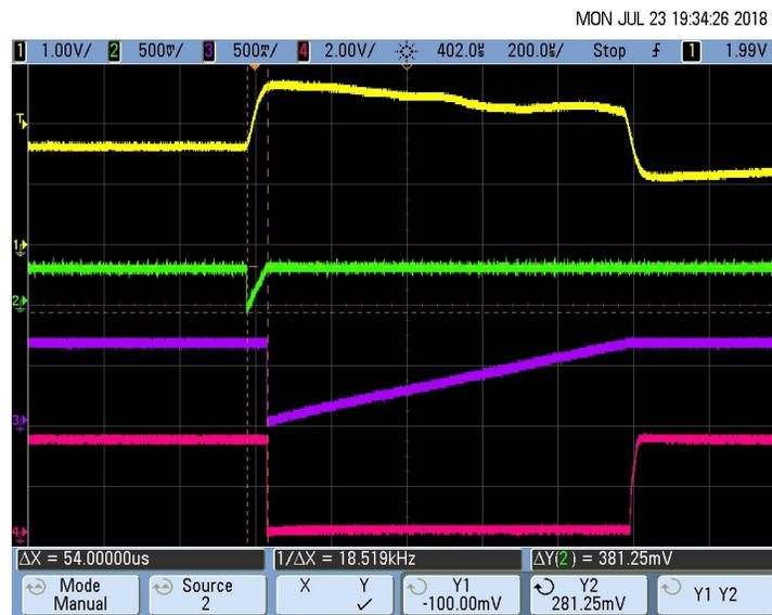
Figure 62. Pacemaker Detection Output (Rise Time  $T_R$ ) for 8-mV, 1-ms Pace Pulse
