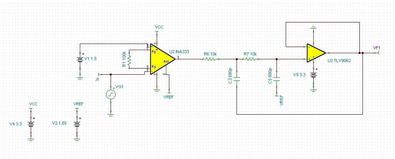
**Figure 13. TINA-TI™ Simulation Circuit of the Low-Pass Filter**
