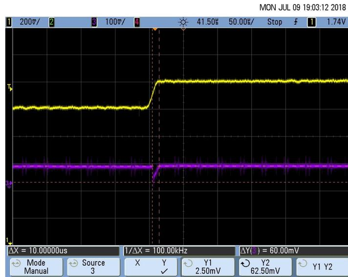
**Figure 46. Rise Time Measurement of the Pace Signal ( $T_R = 10 \mu s$ )**
