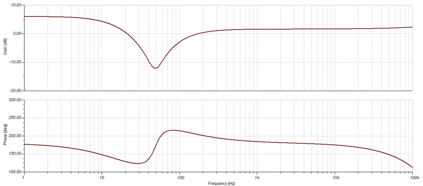
Figure 19. Frequency and Phase Response of the 50-Hz Notch Filter From 1 Hz to 100 kHz
