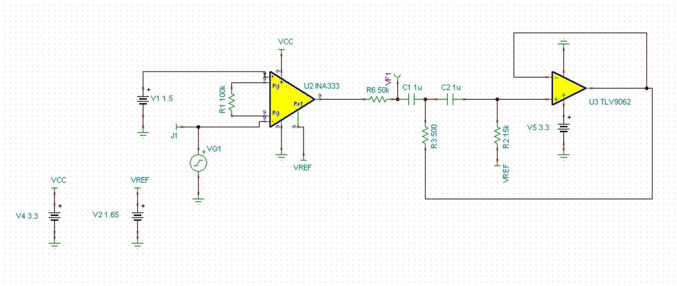
Figure 16. TINA-TI™ Simulation Circuit of the 60-Hz Notch Filter
