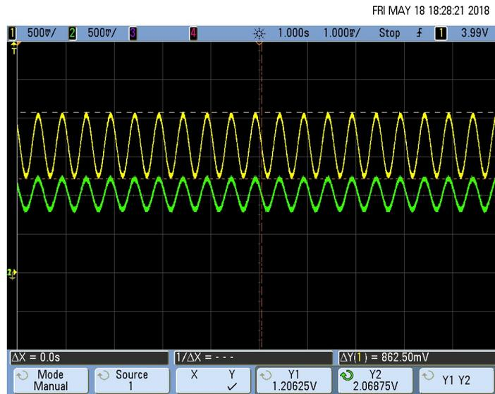
Figure 36. Output Characteristics of Differential to Single-Ended Converter (INA317)
