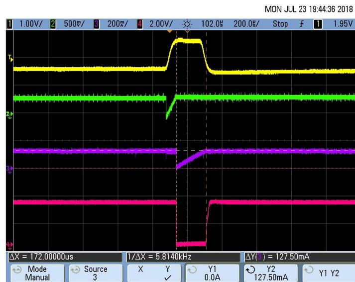
Figure 59. Pacemaker Detection Output (Pulse Duration  $T_P$ ) for 8-mV, 200- $\mu$ s Pace Pulse
