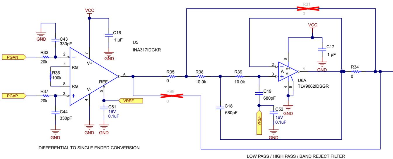
**Figure 12. Low-Pass Filter Schematics for Filter Implementation**
