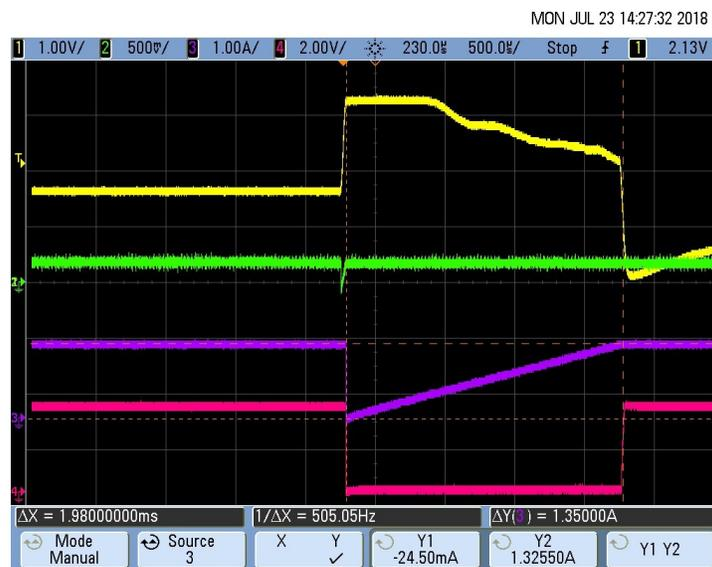
Figure 73. Pacemaker Detection Output (Pulse Duration  $T_D$ ) for 16 mV, 2 ms Pace Pulse
