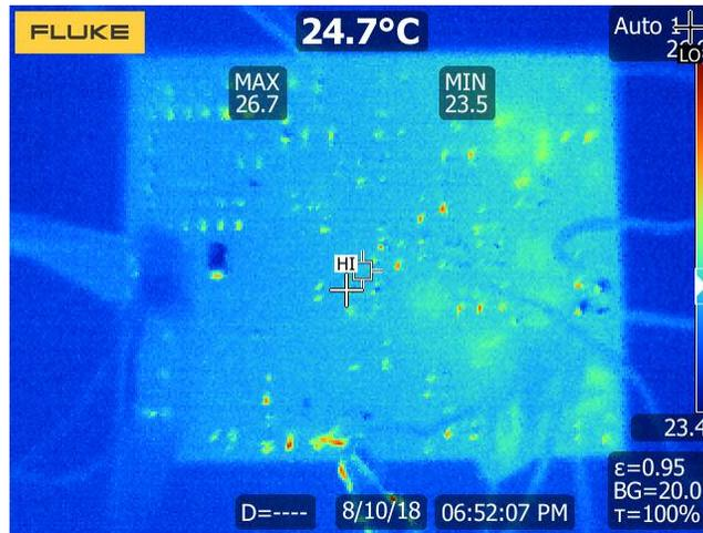
Figure 83. Thermal Image of the Top Section of TIDA-010005
