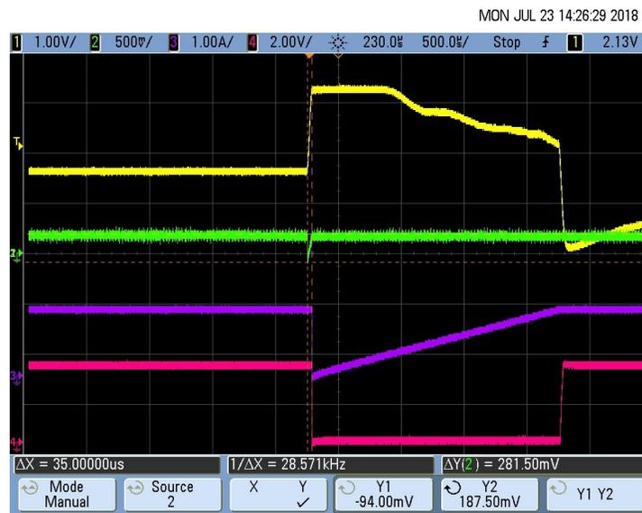
Figure 72. Pacemaker Detection Output (Rise Time  $T_R$ ) for 16 mV, 2 ms Pace Pulse
