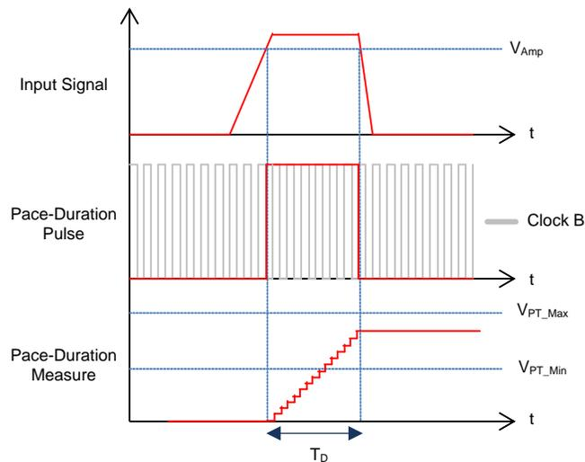
**Figure 6. Pace Duration Pulse Generation and Measurement**
