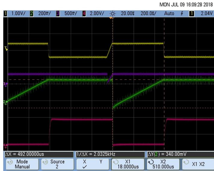
Figure 48. Pulse Duration Measurement of the Pace Pulse ( $T_D = 0.5 \text{ ms}$ )
