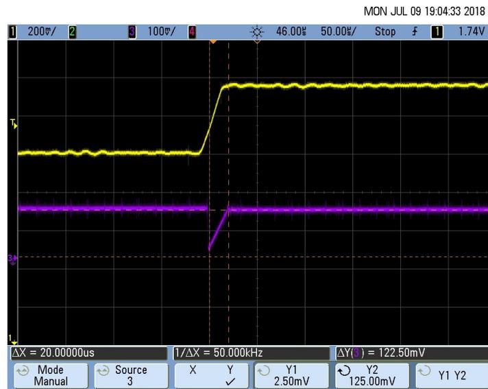
Figure 45. Rise Time Measurement of the Pace Signal ( $T_R = 20 \mu\text{s}$ )
