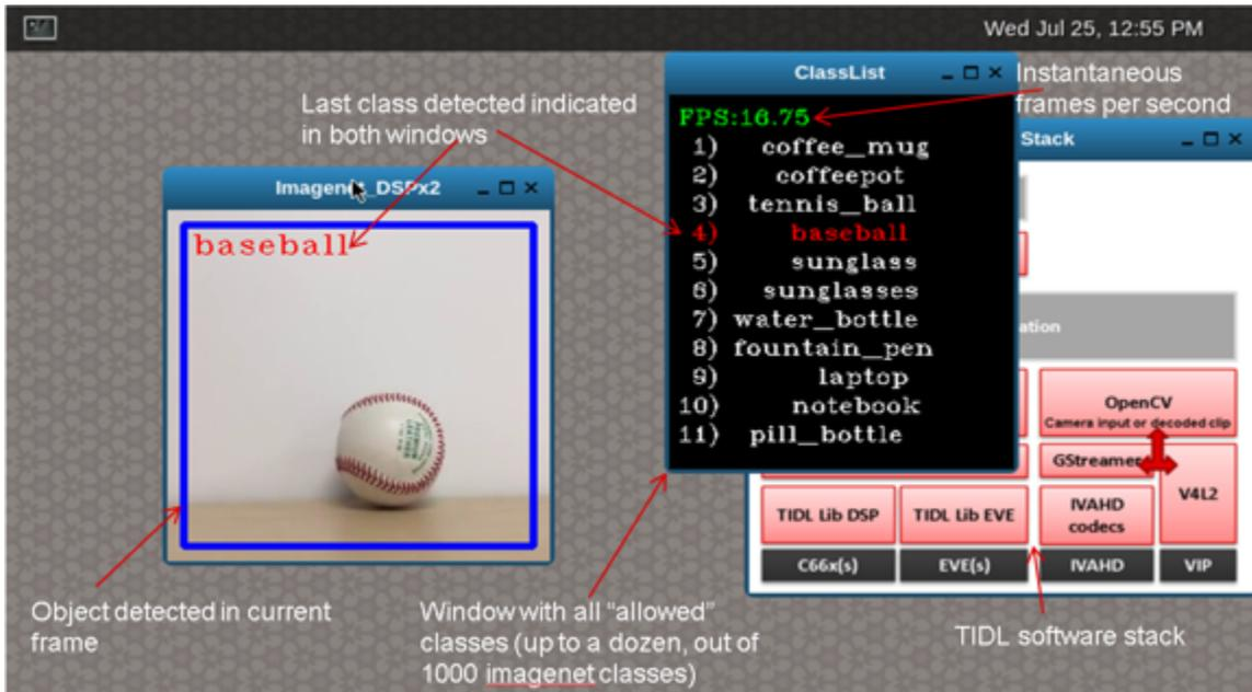
Figure 14. Additional Objects Detected
