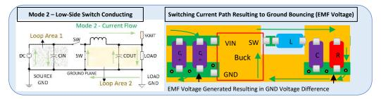
Figure 13. Mode 2 Switching Current
