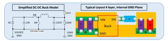
Figure 11. Typical Buck Converter Layout
