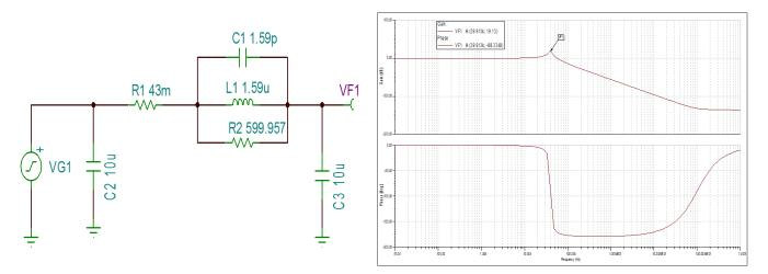
Figure 9. Undamped Filter Response
