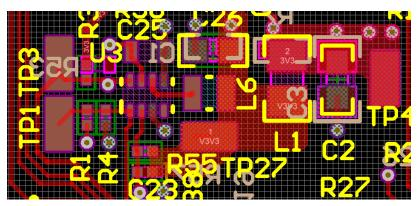
Figure 15. DC/DC Layout Example
