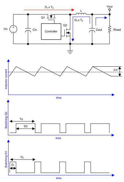
Figure 2. CCM Mode Operation
