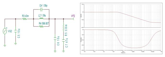
Figure 10. Damped Filter Response
