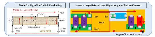
Figure 12. Mode 1 Switching Current
