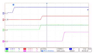
Figure 92. Passive Sequencing 0.1 V, 1.35 V, 3.3 V, and 1.8 V
