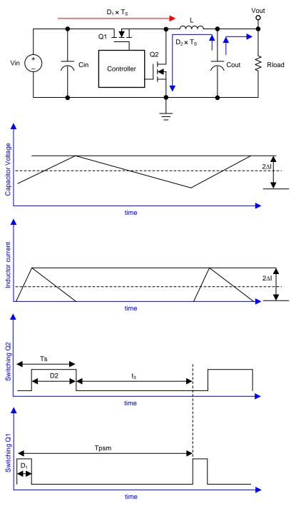
Figure 3. DCM Mode Operation
