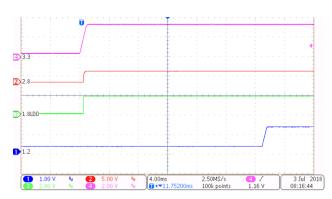
Figure 93. Passive Sequencing 2.8 V, 1.8 V, and 1.2 V
