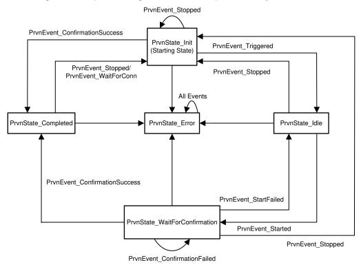
Figure 2-8. Provisioning Task State Machine
