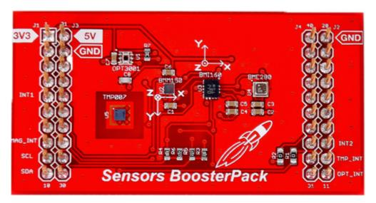
Figure 3-3. BOOSTXL-SENSORS Sensors BoosterPack™ Plug-In Module
