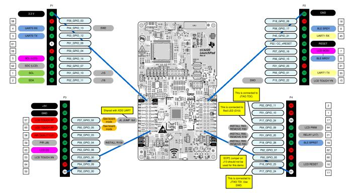
Figure 3-9. TIDM-1020 BLE Provisioning Pin Map
