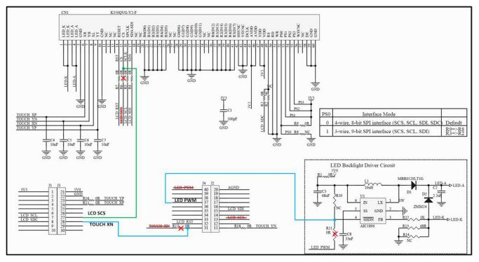
Figure 3-13. Modifications Needed for Kentec QVGA Display BoosterPack™
