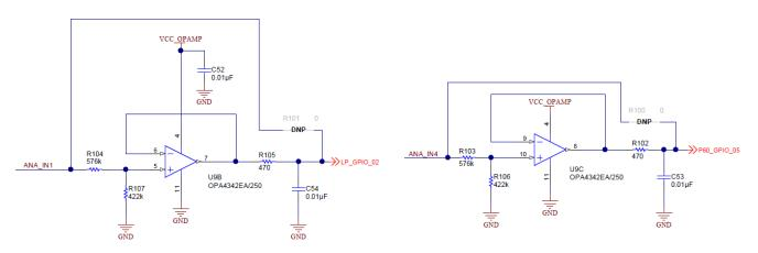
Figure 3-11. Original Circuit for ADC Buffer
