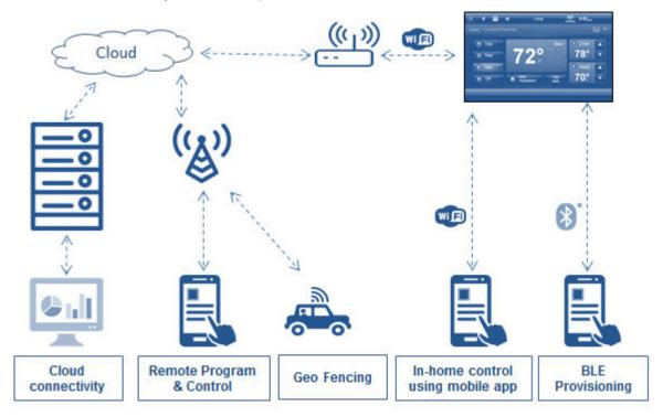
Figure 1-1. Smart-Thermostat System-Level Block Diagram with BLE Provisioning
