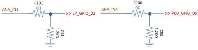
Figure 3-12. Modified Circuit After Modifications
