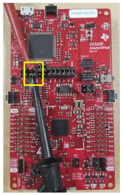
Figure 3-25. Probe Connection for Power Measurement
