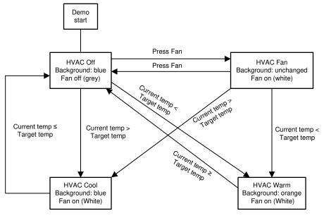
Figure 2-5. State Diagram of HMI Event Flow
