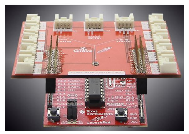
Figure 3-5. Grove Base BoosterPack™ for TI LaunchPad™
