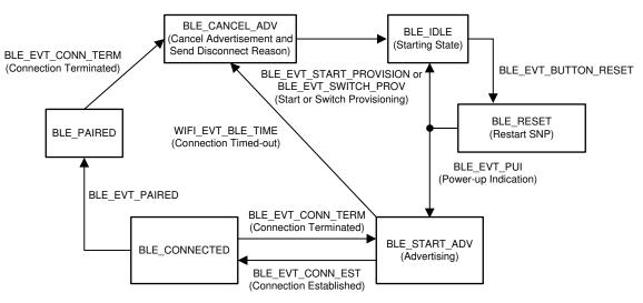
Figure 2-9. BLE Provisioning State Machine
