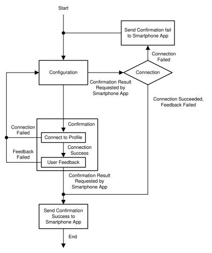
Figure 2-7. Provisioning-Process Flow Chart
