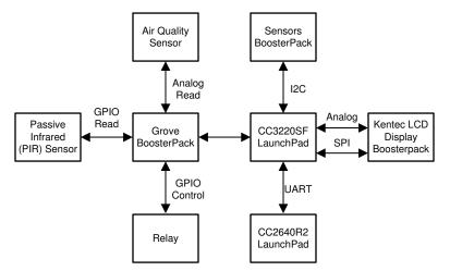
Figure 2-1. TIDM-1020 Block Diagram with BLE Provisioning
