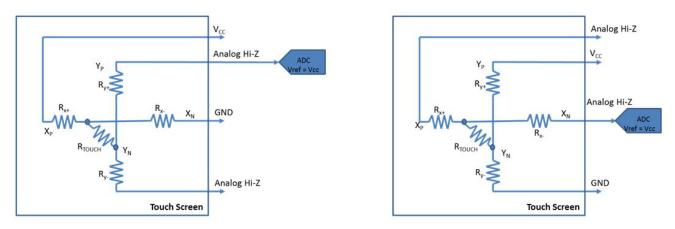
Figure 2-6. Configuration to Read XY Position of Touch Sensor
