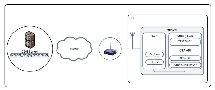
Figure 2-10. OTA System-Block Diagram
