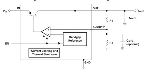
Figure 10. TL5209 Functional Block Diagram
