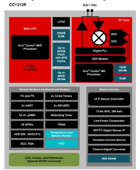
Figure 4. CC1312R Functional Block Diagram
