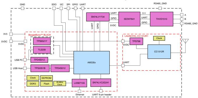
Figure 2. TIDA-010032 Block Diagram
