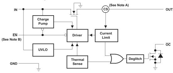
Figure 12. TPS2051B Functional Block Diagram
