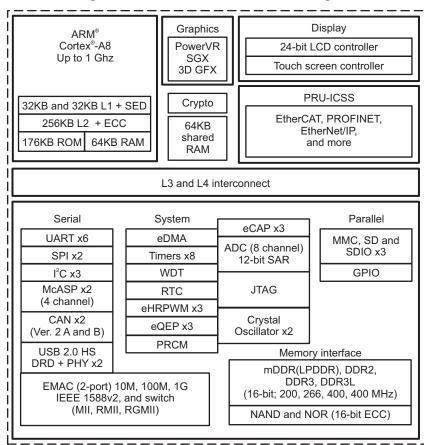
Figure 3. AM335x Functional Block Diagram
