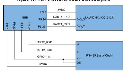
Figure 16. TIDA-010032 Hardware Block Diagram
