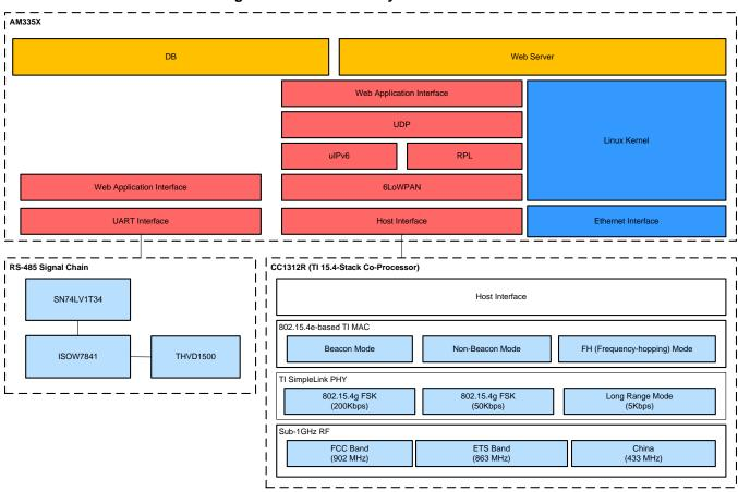
Figure 1. TIDA-010032 System Architecture
