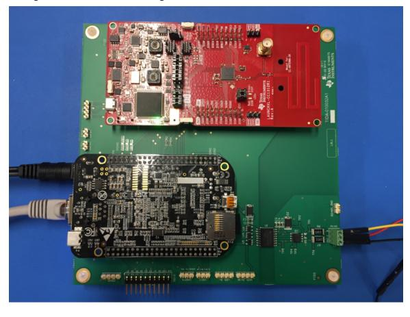
Figure 17. TIDA-010032 Docking Board With BBB and LAUNCHXL-CC1312R1 EVMs
