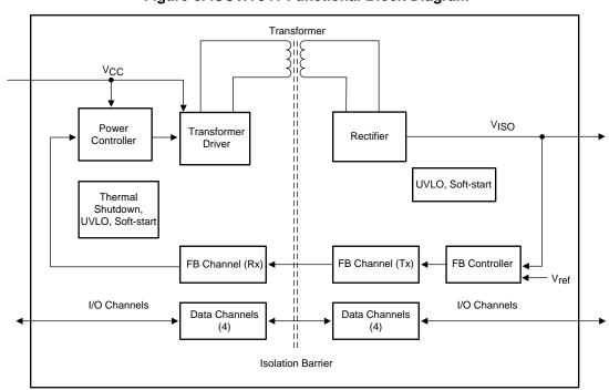
Figure 6. ISOW7841 Functional Block Diagram
