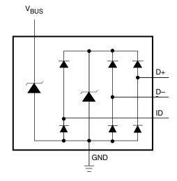
Figure 11. TPD4S012 Functional Block Diagram
