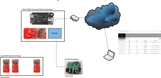
Figure 31. TIDA-010032 Test Setup
