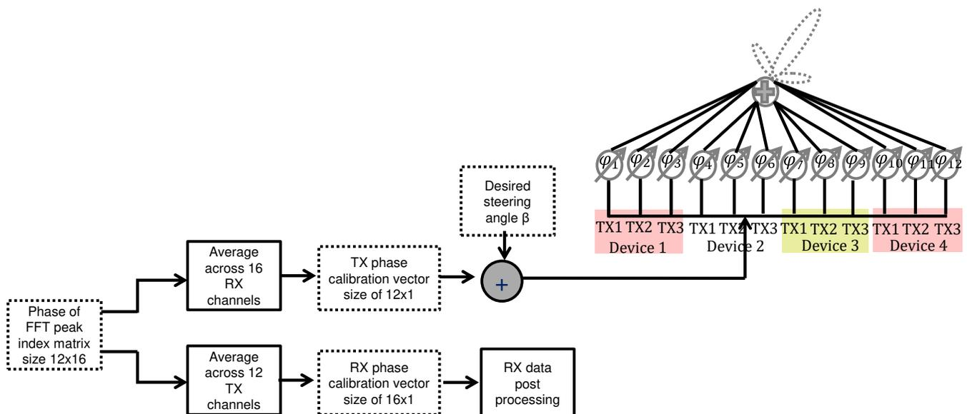
Similarly, the phase across the 12 TX channels is averaged to obtain a phase calibration vector for the 16 RX channels. This is phase only RX calibration assuming that there is no frequency mismatch across the 16 RX channels. The frequency mismatch across 16 RX channels can be captured by collecting calibration data by following these steps.
