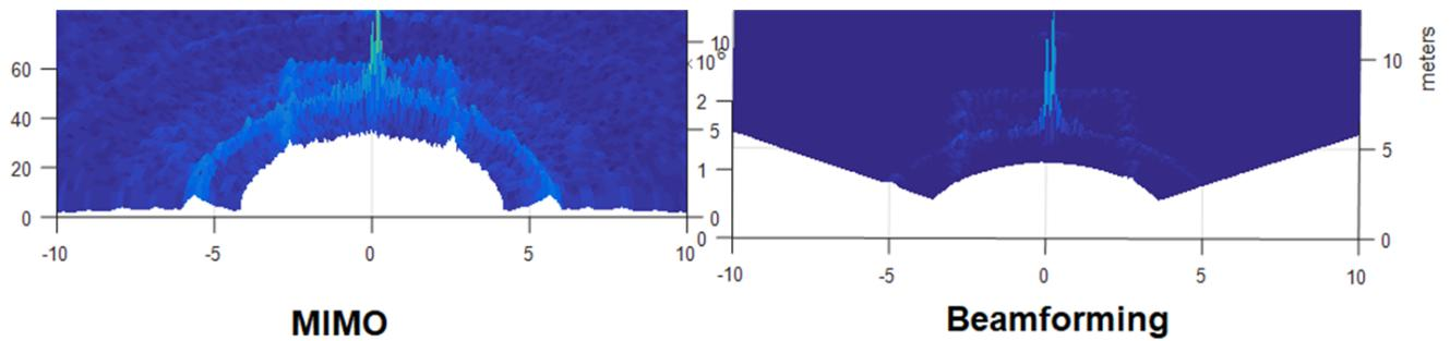
This experiment result proves that the receiver angle resolution in these two operation modes are equivalent since the effective aperture size is the same. Further, the signal SNR in the beamforming is much higher due to the coherent gain in TX beamforming mode. The SNR in MIMO mode can be improved by increasing the chirp integration time.
