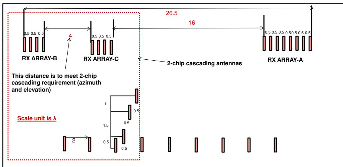
Figure 7. 4-Device Cascade Virtual MIMO Array with 12 TX and 16 RX
