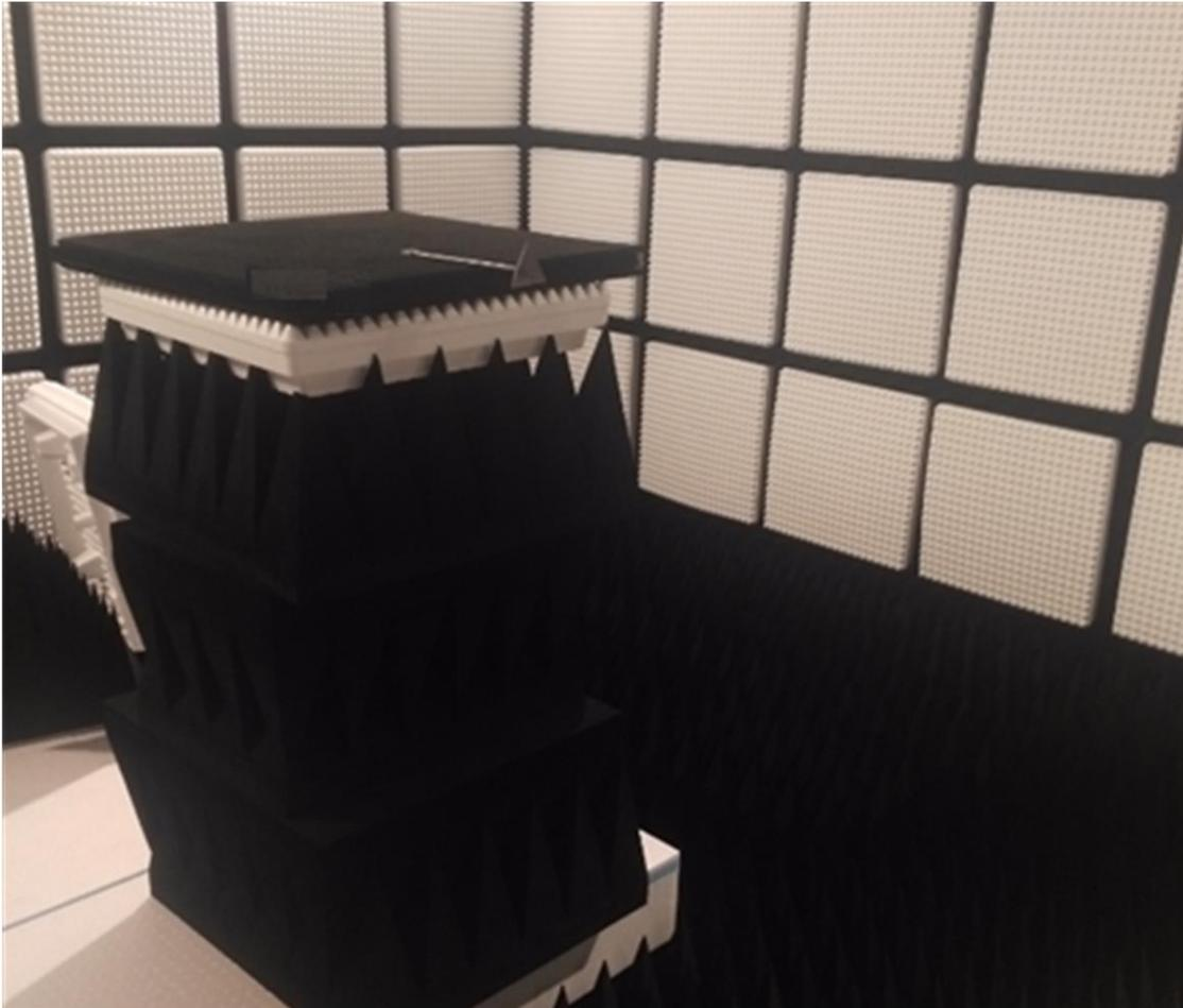
When the corner reflector is placed at the center position, a few frames of raw ADC data needs to be collected by using the example script provided in the mmWave Studio release. During the data collection, turn on 12 TX in a TDM MIMO mode and all 16 RX channels are on at the same time.
