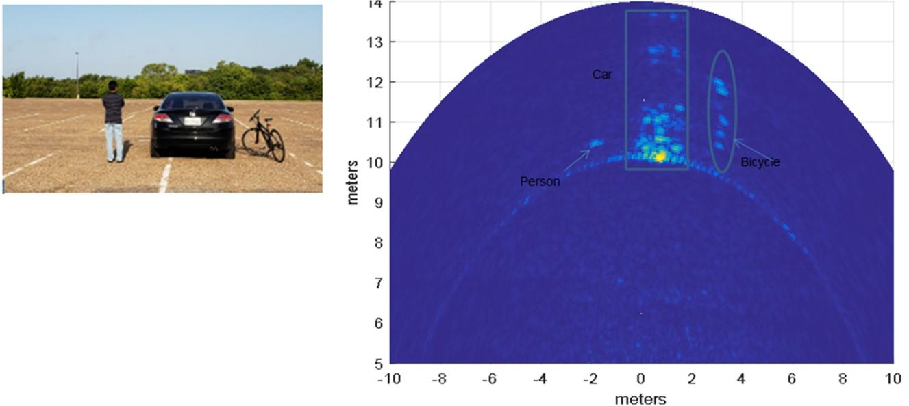
**Figure 26. Bicycle and Person 1.0 Meter (left) and 0.5 Meter (right) Away From Vehicle**
