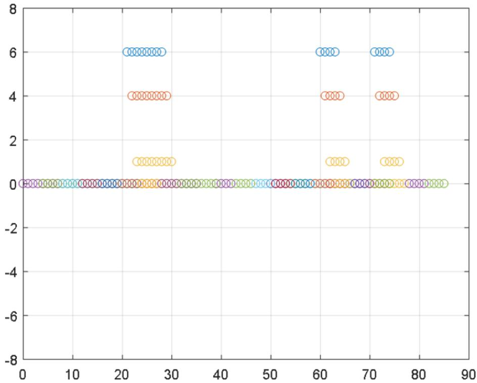
Figure 8. 2-Device Cascade Virtual MIMO Array with 6 TX and 8 RX
