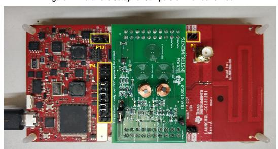
Figure 21. Hardware Setup for Jumpers on the LaunchPad
