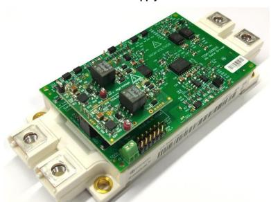
Figure 20. LM5180-Q1 Based Bias Supply Connected to the Power Stage
