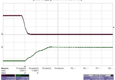
Figure 60. Power-Down Waveform of the -9-V Rail With  $V_{IN}$  = 12 V and no Load (Bias Supply With TPS40210-Q1)
