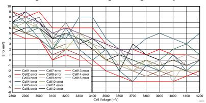
Figure 7. Cell 1–15 Voltage Sensing Accuracy
