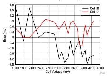
Figure 8. 16th and 17th Cell Voltage Sensing Accuracy at 25°C
