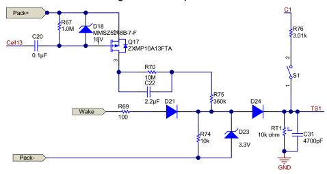
Figure 3. Wake-Up Circuit
