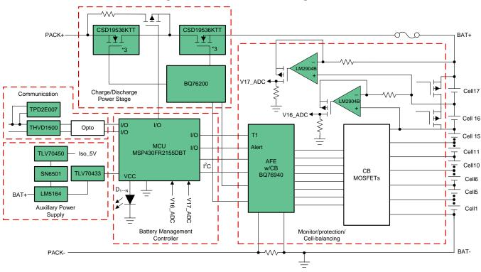
Figure 1. TIDA-010074 Block Diagram
