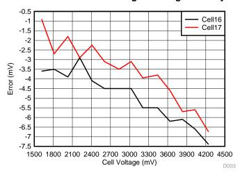
Figure 10. 16th and 17th Cell Voltage Sensing Accuracy at 0°C
