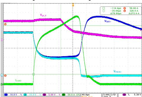
Figure 19. Short-Circuit Discharge Protection
