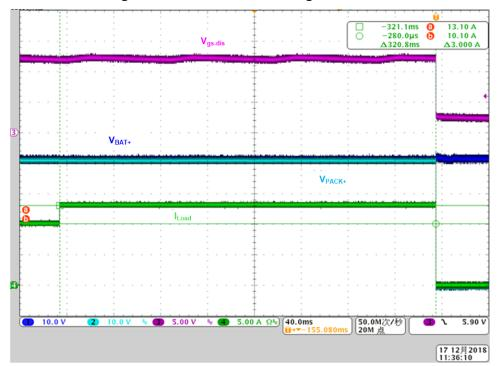
Figure 18. Overcurrent Discharge Protection
