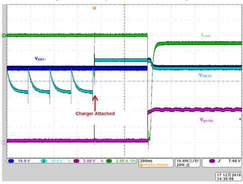
Figure 16. Standby Scenario 1 Detect Charger
