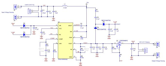
Figure 3. TPS61089 Boost Converter
