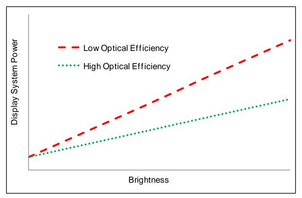
Figure 6-1. High Optical Efficiency Lowers System Power as Brightness Increases
