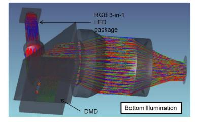
Figure 3-6. Example Optical Designs with Side and Bottom Illumination Orientations
