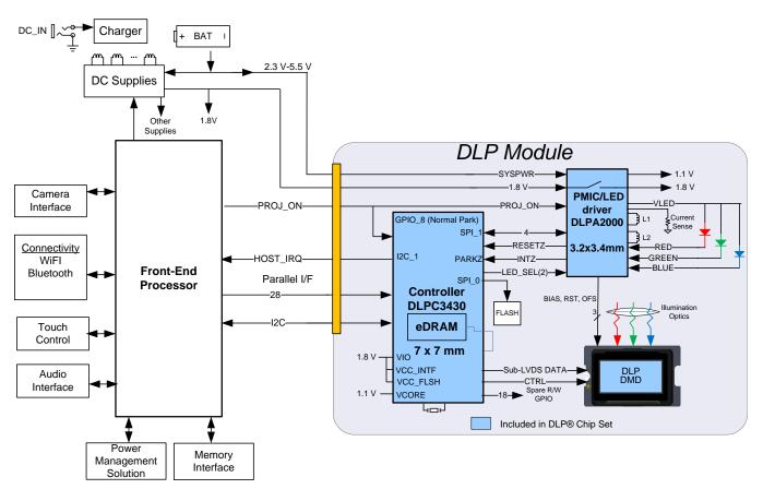
Figure 4-2. Example System Block Diagram
