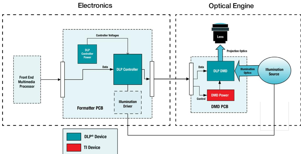
Figure 5. Typical DLP technology display system block diagram.
