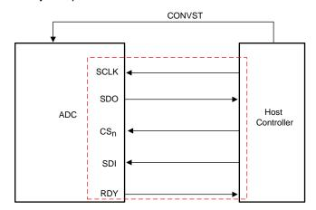
Figure 2. Pins Used by the multiSPI Digital Interface
