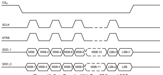
Figure 12. Data Transfer With Two SDOs and DDR
