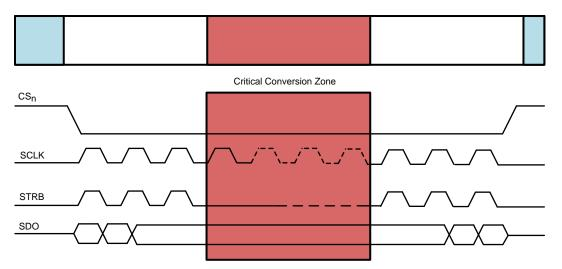
Figure 10. Closer Look at Latency 1 Operation Through Critical Silent Zones
