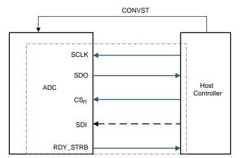
Figure 5. Signals Used for Source Synchronous Data Transfer
