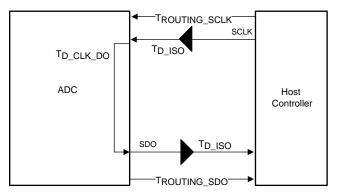
Figure 4. Data Transfer Delays Encountered in a Host or ADC System
