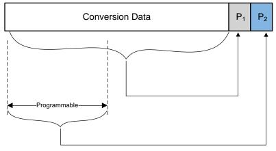
Figure 15. Parity Bits Computation Based on the Conversion Data
