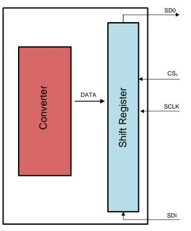
Figure 13. multiSPI Digital Interface SDI to SDO Feed-Through Shift-Mode Feature
