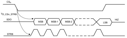
Figure 7. Source Synchronous Data Transfer With an Internal Clock Source Mode for STRB Generation
