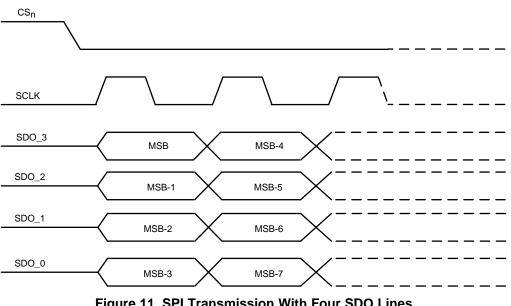
Figure 11. SPI Transmission With Four SDO Lines
