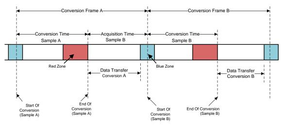
Figure 3. Conversion and Data Transfer Windows Present Within Each Frame
