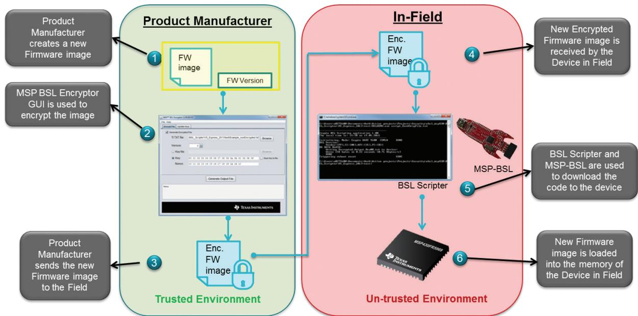
Figure 3: Crypto-Bootloader tools in in-field firmware updates flow
