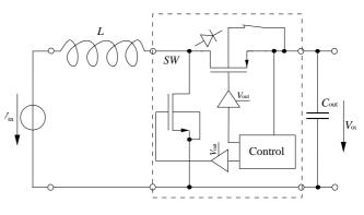
Fig. 3. Schematic of the converter in boost mode.
