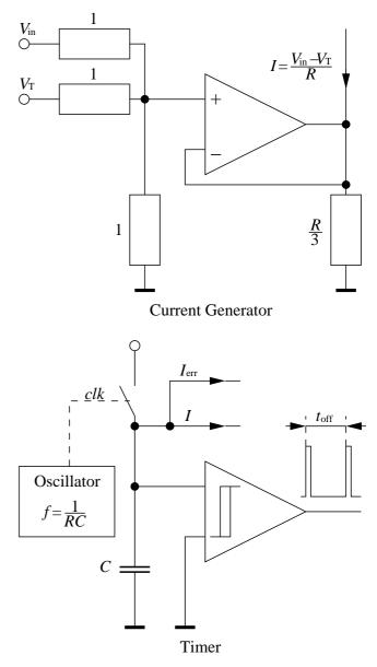
Fig. 8. Controller scheme for down mode.
