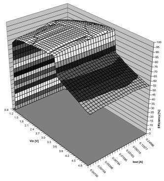
Fig. 10. Efficiency for  $V_{out} = 5.5V$  with power save mode enabled.
