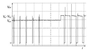
Fig. 7. Signal at SW at the changeover from boost mode (left) to down mode.
