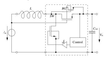
Fig. 5. Schematic of the converter in down mode.
