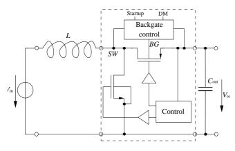
Fig. 2. Blockdiagram of the boost converter with down conversion capability.
