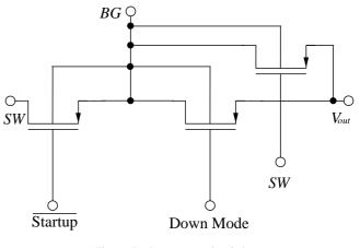
Fig. 6. Back-gate control switches .
