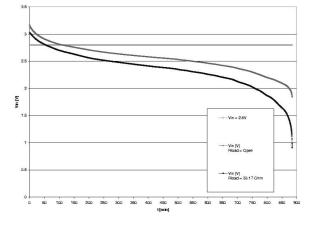
Fig. 1. Discharging of two alkaline cells in series at a boost converter input.
