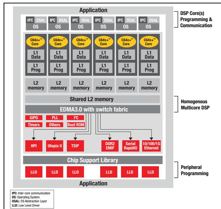
▲ Figure 2: Multicore software framework for the TMS320C6472 processor
