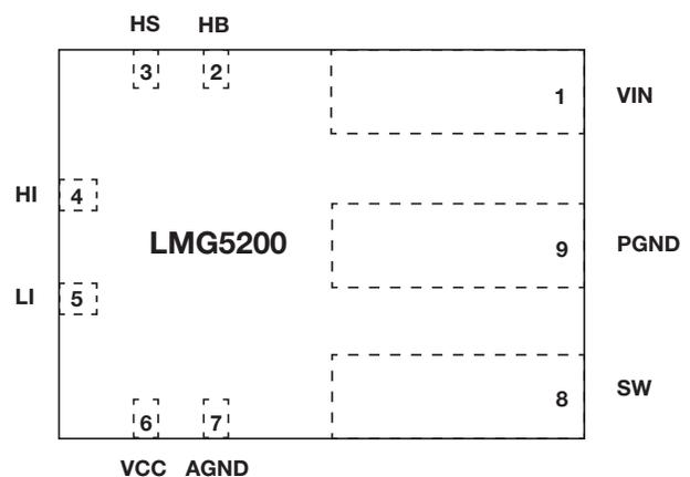
**Figure 1.** Top-down view of a GaN FET power stage device, showing pin-out.
