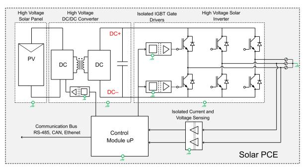
Figure 3. System block diagram of a transformer-based solar power conversion system.
