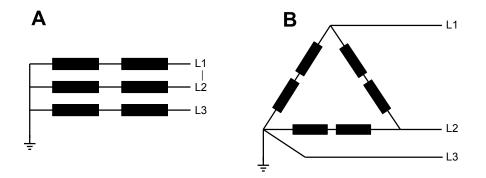
Figure 4. (a) A star-earthed TN system that is neutral-earthed; and (b) a corner-earthed TN system where one phase is earthed.
