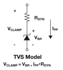
Figure 5. Electrical model of conventional TVS clamps.
