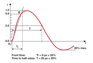
*Figure 3.* Waveform of a short-circuit current at the output of the CWG.
