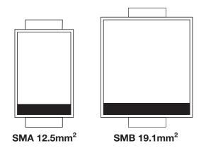
*Figure 1.* Standard packages for discrete TVS surge protection diodes.
