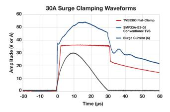
*Figure 8.* 8/20µs surge clamping of a Flat-Clamp diode vs. a conventional TVS diode.
