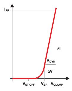
Figure 4. Standoff, breakdown and clamp voltage.
