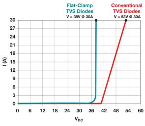
**Figure 7.** DC  $I_{\mathbb{N}}$ - $V_{\mathbb{N}}$  curves of a Flat-Clamp diode vs. conventional TVS diodes.
