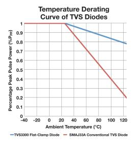
*Figure 13. Temperature derating curve of the TI Flat-Clamp family.*
