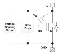
Figure 6. Flat-Clamp technology functional block diagram.
