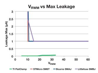
*Figure 12. V*<sub>*RWM</sub> vs. maximum leakage current for the TI Flat-Clamp family vs. conventional TVS diodes.*</sub>
