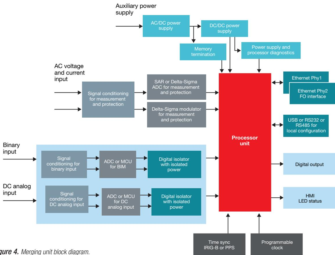
**Figure 4.** Merging unit block diagram.
