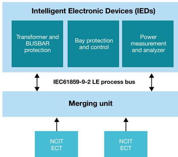
**Figure 5.** A merging unit interfaced to non-conventional instrument transformers.
