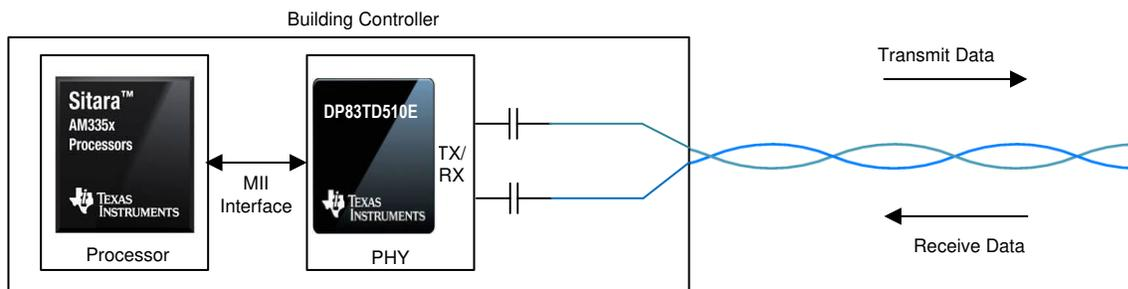
**SPE Interface for 10 Mbps Using the DP83TD510E**
