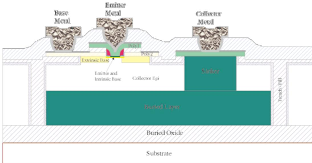
**Figure 1: VIP10 Transistor Cross Section**
