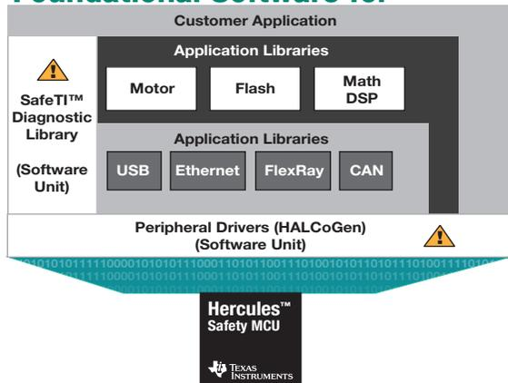
Figure 1. Software Stack built on top of Hercules™ Safety MCU
