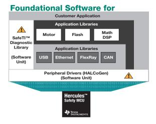
Figure 1. Software Stack built on top of Hercules<sup>™</sup> Safety MCU **Figure 1** shows a typical software stack. The customer application is developed on top of lowlevel drivers and application libraries. Typically the software components of the software stack are developed by different vendors, which are then integrated by the system developers into a system or application.
