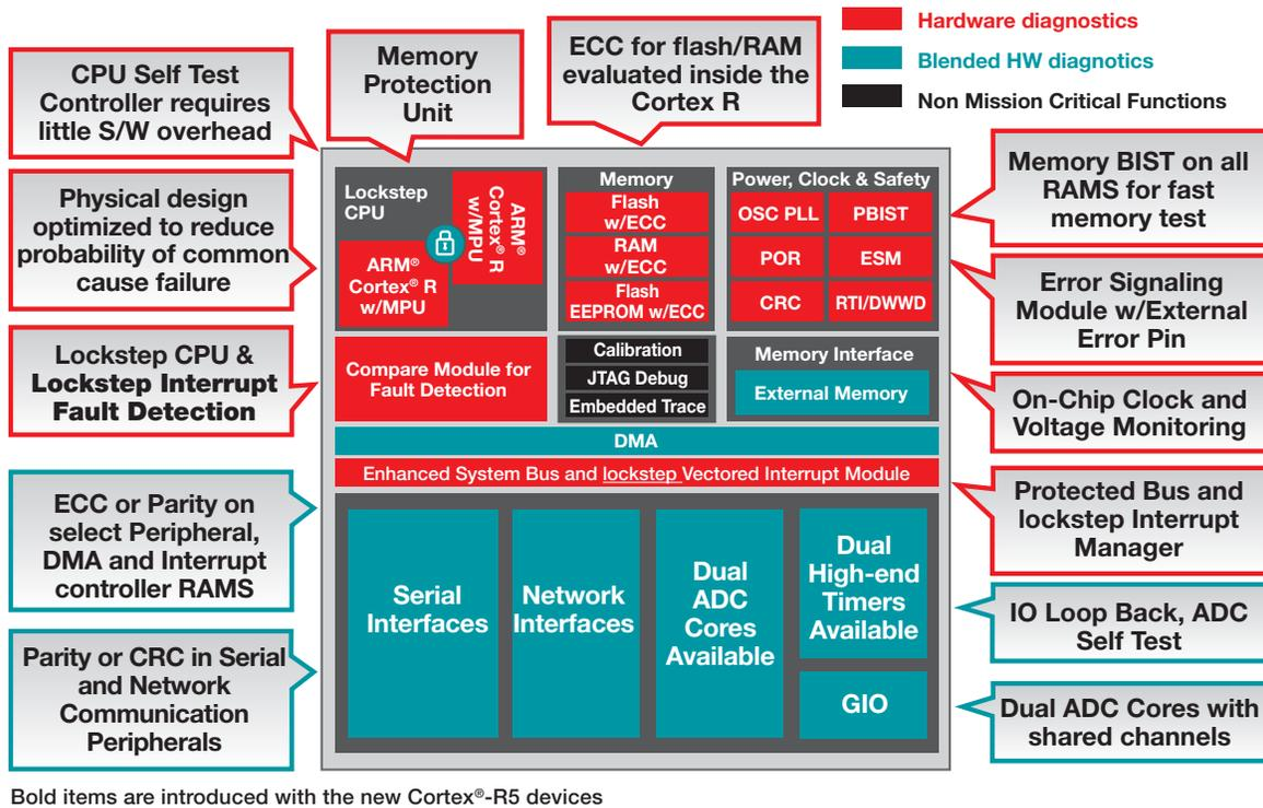
Figure 1: Hercules MCU diagnostic features
