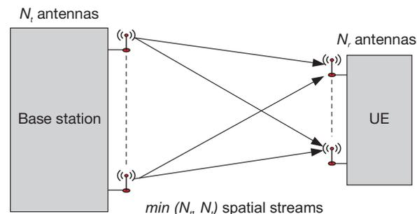
Figure 2. Illustration of a MIMO system between a base station and UE.
