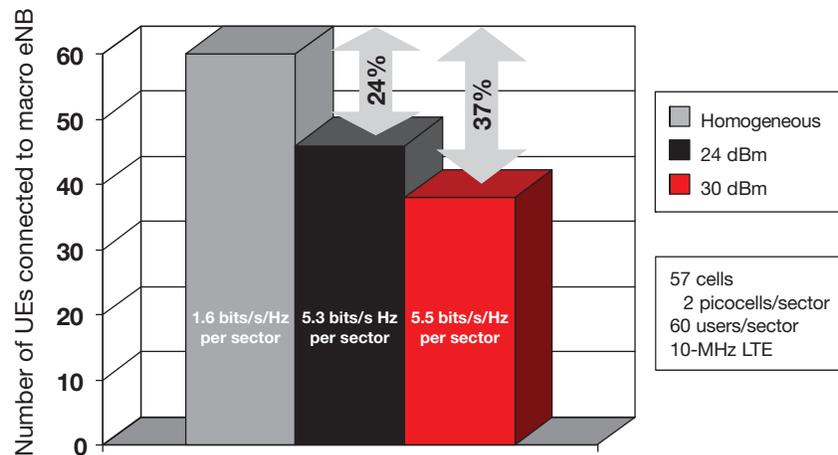
Figure 3. Spectral efficiency improvements with small cells.
