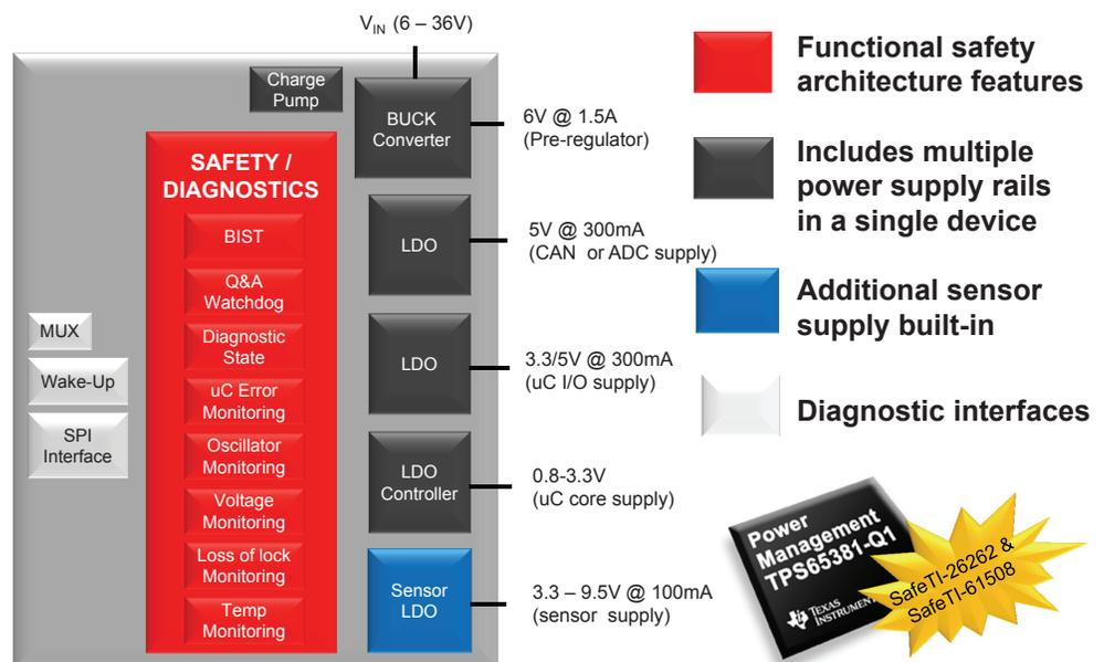
Figure 7. The TPS65381-Q1 multi-rail safety PMIC
