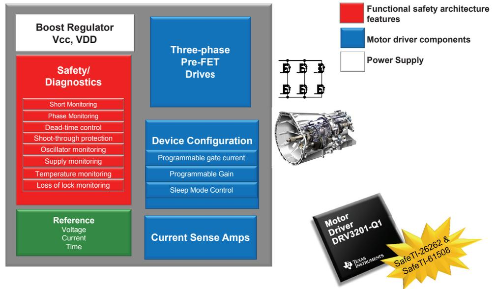
Figure 8. DRV3201-Q1 safety motor driver
