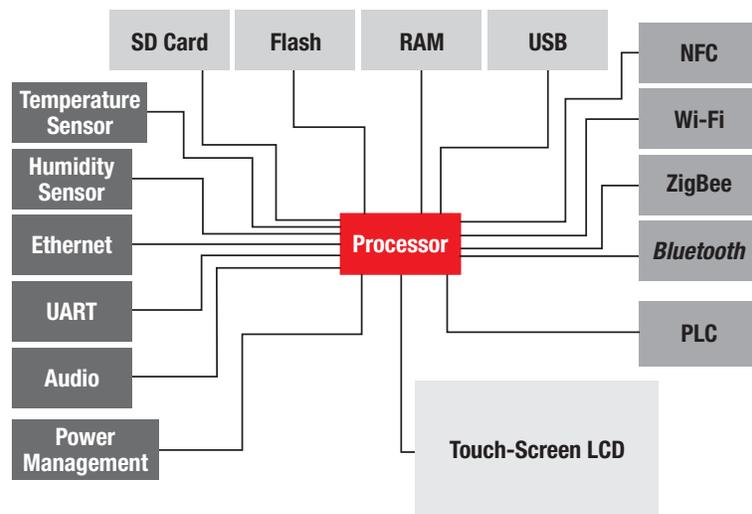
**Figure 1. Smart thermostat architecture**
