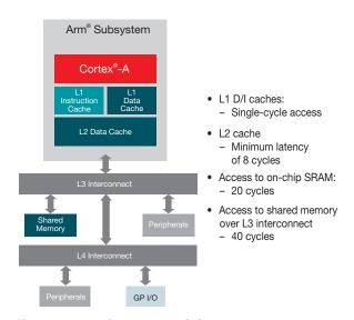
Figure 1. A typical Cortex-A-based SoC general-purpose processing architecture.
