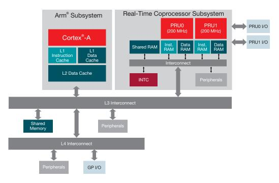
Figure 2. A general-purpose core supplemented with real-time co-processors.
