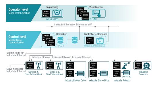
Figure 6. Factory automated systems with AMIC110.
