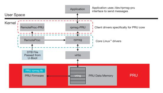
Figure 5. Sitara Arm/PRU software architecture.
