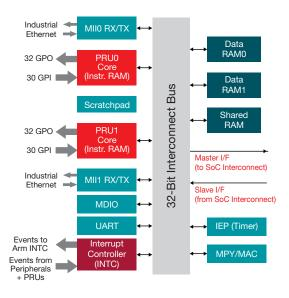
Figure 3. The TI Programmable Real-Time Unit (PRU) subsystem.
