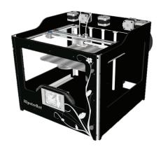
Figure 7. Sitara AM335x with Arm Cortex-A8 core and PRU running a 3D printer.
