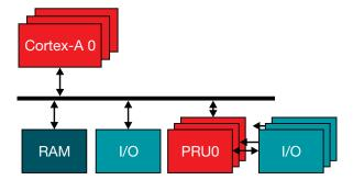
Figure 4. Base Sitara architecture with Arm cores and PRUs.
