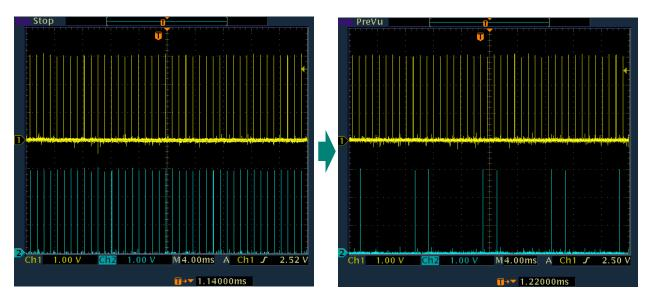
*Figure 1.* These screen captures illustrate two oscilloscope traces. The top (yellow) trace tracks a timer that triggers every 1 ms for use as a comparison against the bottom (blue trace), which tracks triggering for a timer used to generate a 1-ms system tick for TI-RTOS. In the left-side screens, these two traces line up as expected. In the right-side screens, TI-RTOS tick suppression is enabled, resulting in fewer interrupts, as they occur only when work is actually scheduled for execution.
