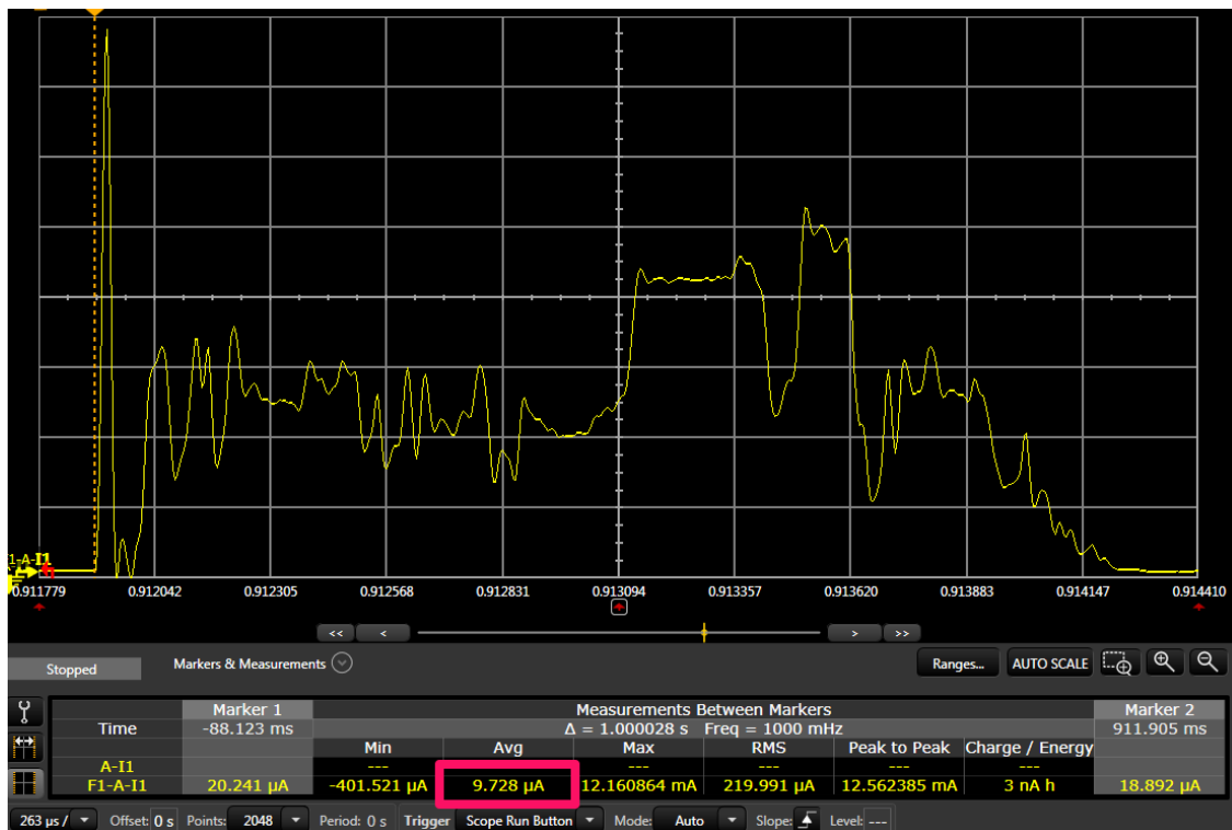
Figure 3. This current-consumption profile highlights the < 10 \mu A average for maintaining a Bluetooth low energy connection with a 1-s connection interval. The device wakes from standby and the radio powers up to do a receive operation, followed by a transmit operation. The device then quickly transitions back to standby. Note the very low current used in standby mode.
