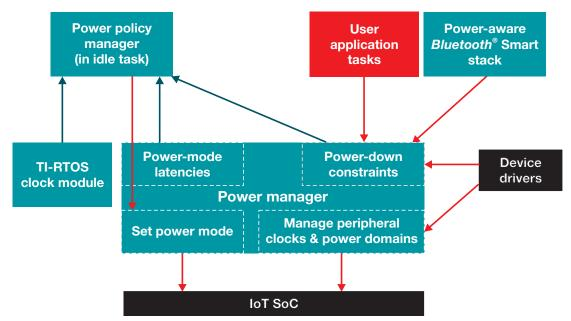
*Figure 2.* The TI-RTOS power manager delivers significantly lower power performance with minimal user intervention. Key system components such as drivers and stacks are power-aware and inform the power manager when it is safe to aggressively power down. The power policy manager combines this information with the knowledge of upcoming events to decide which power state to select.
