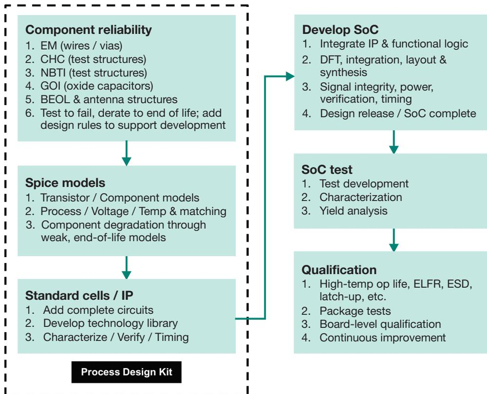
Figure 3: Design for intrinsic reliability process flow
