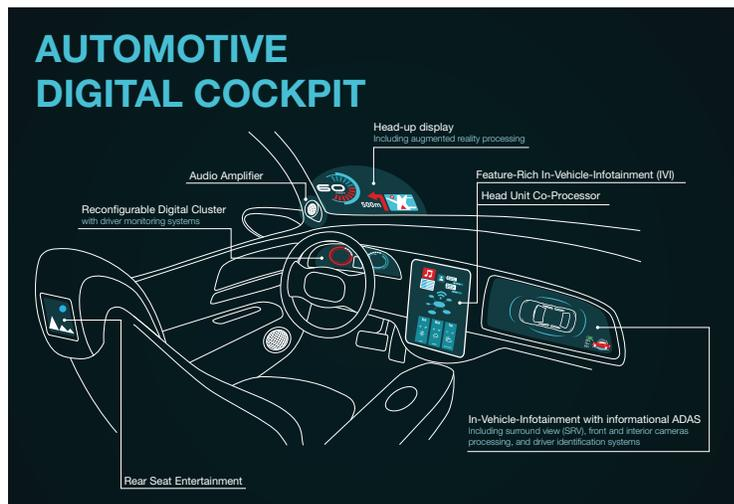
Figure 5. Digital cockpit applications supported by TI "Jacinto" processors.
