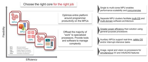
Figure 6. Heterogeneous architecture: one size does not fit all.
