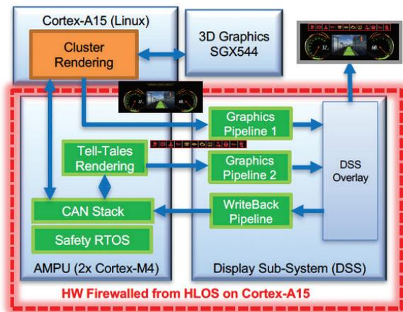
Figure 6. Jacinto 6 safety architecture based on AMPU.
