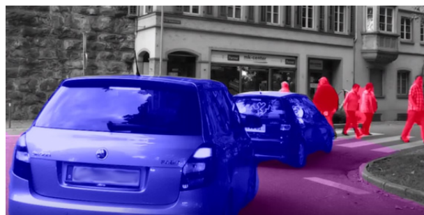
Figure 2. Semantic segmentation using TIDL on a TDA2 SoC.
