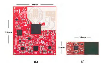
**Figure 1.** Comparing a 60-GHz 55-Mm-by-55-Mm TI mmWave Evaluation Board with External Antenna; and the New 15-Mmby-36-Mm Evaluation Board Design with TI's mmWave AoP Sensor.
