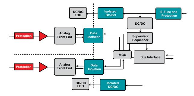
Figure 1. PLC with isolation
