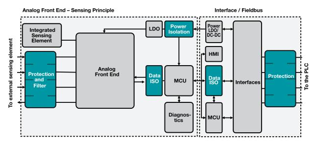
Figure 2. Sensor with isolation
